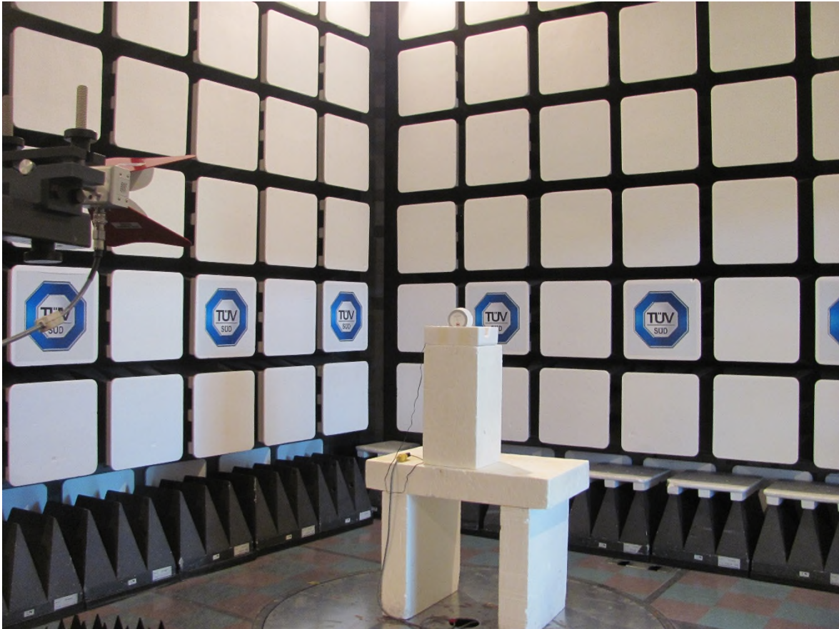
Figure 3 – Radiated Emissions Setup – Photo 3
