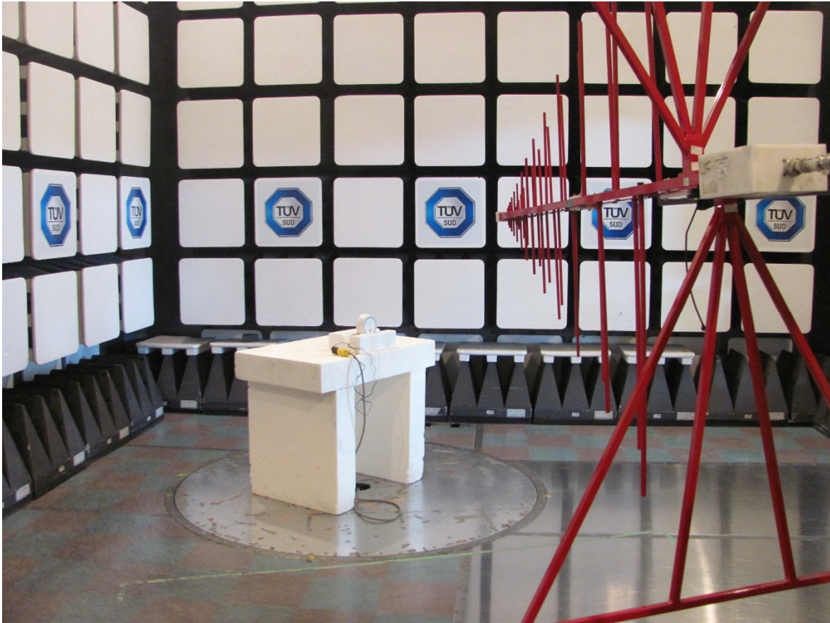
Figure 2 – Radiated Emissions Setup – Photo 2
