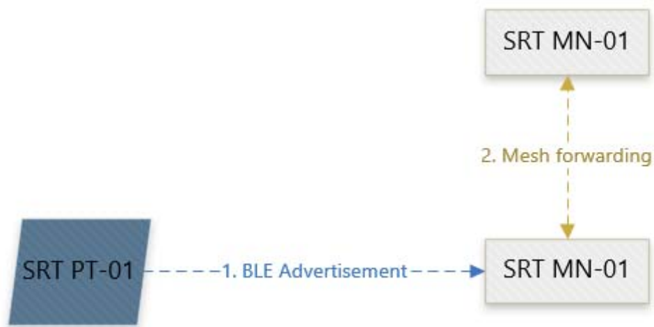
Figure 2- Tag and Meshnode communication pattern
