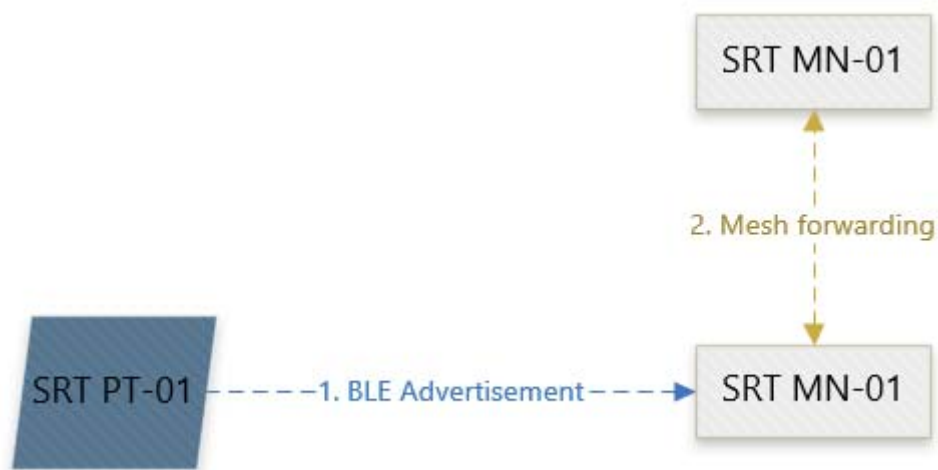
Figure 2- Tag and Meshnode communication pattern
