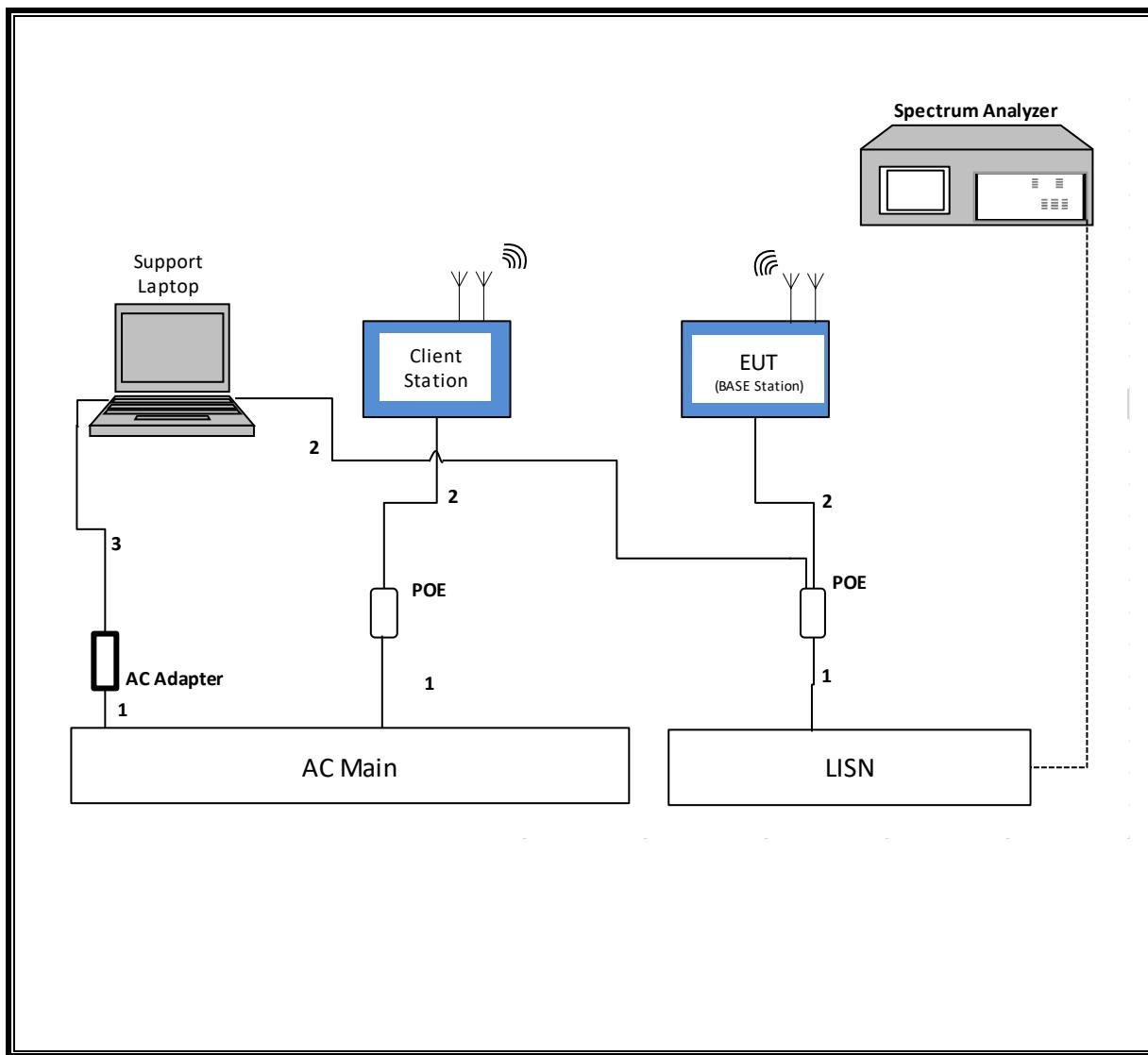
**SETUP DIAGRAM AC LINE CONDUCTED TESTS - CLIENT**
