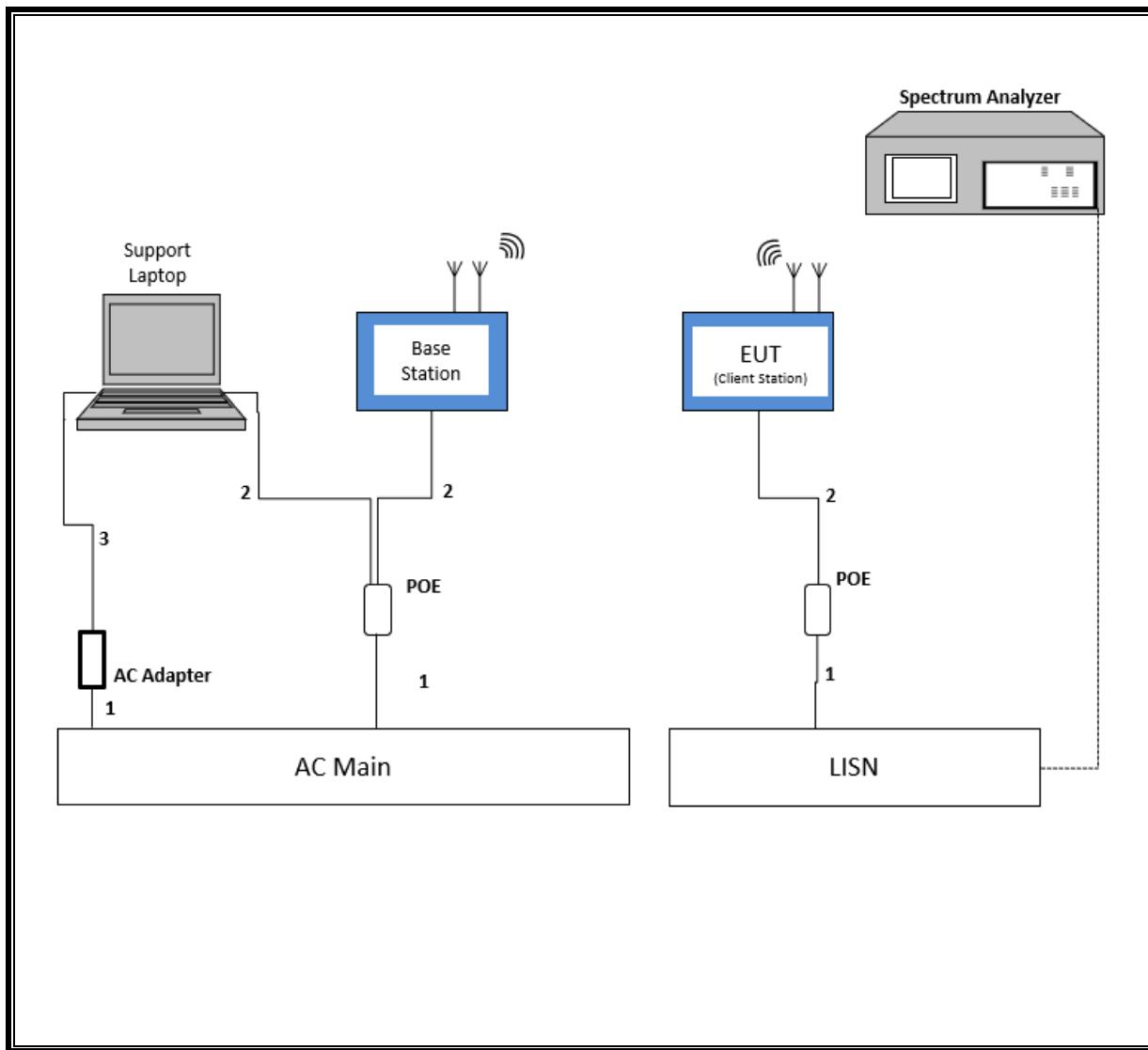
**SETUP DIAGRAM ANTENNA PORT CONDUCTED TESTS**
