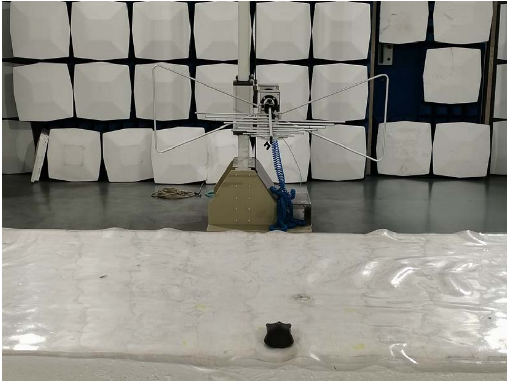
Radiated emission test view
