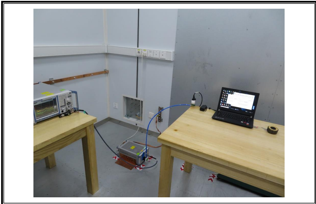
CONDUCTED EMISSION TEST FOR AC POWER PORT MEASUREMENT SETUP
