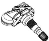
1.2 Before the transmitter is installed, the rim around the hole must be cleaned with a cloth.
