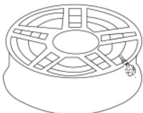
1.5 Lock the rim on the tyre changer. (If the mounting head of the tyre changer is positioned at 12 o'clock, then the valve should be at the 7 o'clock position.) Apply lubricant on both the tyre bead and rim. Mount the lower tyre bead on the rim. Ensure that the tyre bead does not touch the electronic module during mounting.
