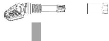
1.4 Place nut<sup>④</sup> on the valve stem, and tighten with 5 Nm (44 inch pounds) torque.
