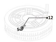
1.7 Apply soapsuds on the valve tip. If no leakage is found, put on the valve cape. If unsuccessful, try again.
