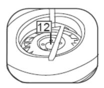
2.4 Final inspection: Visually inspect the rim, valve stem and electronic module to ensure no damage has occurred.
