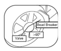
2.2 Firmly fix the wheel on the turntable clamps. (If the mounting head of the tyre changer is positioned at 12 o'clock, then the valves stem should be at the 11 o'clock position.) Apply lubricant to both tyre bead and rim, and then remove the upper tyre bead.
