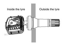
1.4 Place the Self-lock Screw<sup>®</sup> on the valve stem, and tighten with 5 Nm (44 inch pounds) torque.
