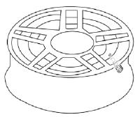
1.5 Lock the rim on the tyre changer. (If the mounting head of the tyre changer is positioned at 12 o'clock, then the valve should be at the 7 o'clock position.) Apply lubricant on both the tyre bead and rim. Mount the lower tyre bead on the rim. Ensure that the tyre bead does not touch the electronic module during mounting.
