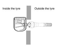
1.4 Place the Self-lock Screw<sup>©</sup> on the valve stem, and tighten with 5 Nm (44 inch pounds) torque.
