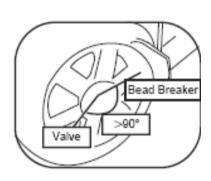
2.2 Firmly fix the wheel on the turntable clamps. (If the mounting head of the tyre changer is positioned at 12 o'clock, then the valves stem should be at the 11 o'clock position.) Apply lubricant to both tyre bead and rim, and then remove the upper tyre bead.
