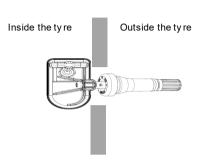
1.4 Place the Self-lock Screw<sup>①</sup> on the valve stem, and tighten with 5 Nm (44 inch pounds) torque.
