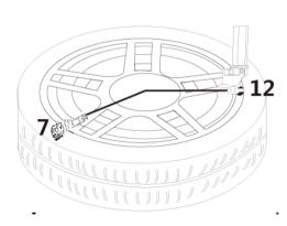
1.6 Mount the upper tyre bead the same way. (If the mounting head of the tyre changer is positioned at 12 o'clock, then the valve should be at the 5 o'clock position.) Inflate the tyre to nominal pressure.
