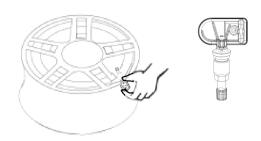
1.3 Take off the nut<sup>®</sup>, insert the valve stem through the rim hole from inside.
