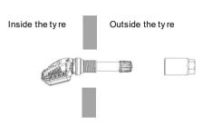
1.4 Place  $\operatorname{nut}^{\scriptsize{\textcircled{\tiny \$}}}$  on the valve stem, and tighten with 5 Nm (44 inch pounds) torque.
