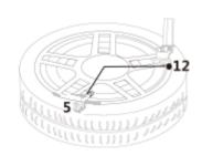
1.7 Apply soapsuds on the valve tip. If no leakage is found, put on the valve cap 6. If unsuccessful, try again.
