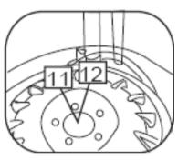
2.3 Use the same procedure to dismount the lower tyre bead. (If the mounting head of the tyre changer is at the 12 o'clock position, then the valves stem should also be at the 12 o'clock position.)
