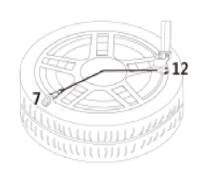
1.6 Mount the upper tyre bead the same way. (If the mounting head of the tyre changer is positioned at 12 o'clock, then the valve should be at the 5 o'clock position.) Inflate the tyre to nominal pressure.
