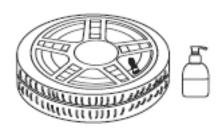
1.8 Dynamically balance the wheel before it is placed back on the vehicle.
