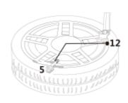
1.7 Apply soapsuds on the valve tip. If no leakage is found, put on the valve cape. If unsuccessful, try again.
