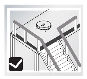
Anti-drop sensors prevent A980 from tubling down stairs and steep drops. They may work less effectively if dirty or used on reflective/ very dark-colored floors. It is recommended to apply the Boundary Strips to block off areas where A980 may fall.
