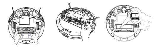
2. Clean the Rolling Brush. Cut down the hair winded in the Rolling Brush with the knife of Cleaning Tool.
