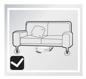
Keep A980 away from spaces lower than 3 inches to prevent A980 from getting stuck. If necessary, place a barricade to block off the area or elevate your appliance.
