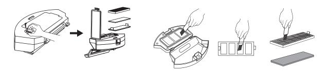
2. Put the filters back together in the Dust Bin.
