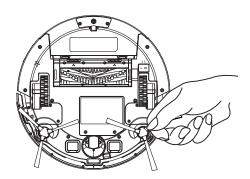
5. Turn on the Main Power Switch at the bottom of Robot. After Robot says "I am ready now" it is ready for use.
