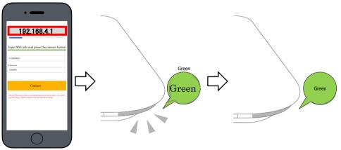
If the lamp turnes red, it indicates SmartMat is not connected to the internet.
