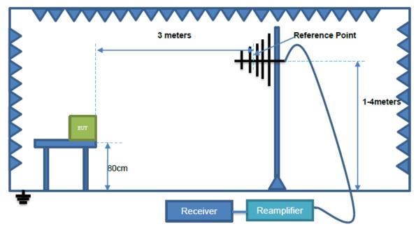
Radiation Test (30MHz - 1GHz)
