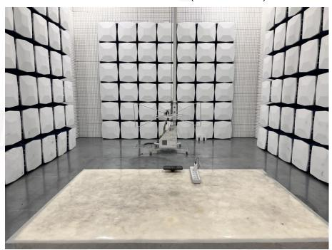
Radiated band emission (9KHz-30MHz):
