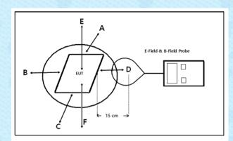
Note: As bottom point is not required to test for desktop devices
