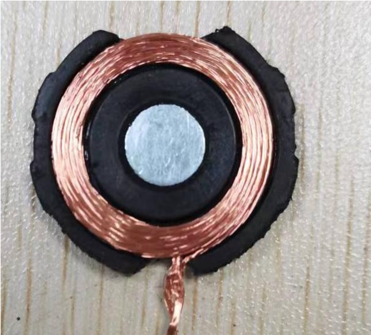
Antenna type: Inductive loop coil Antenna, 0dBi
