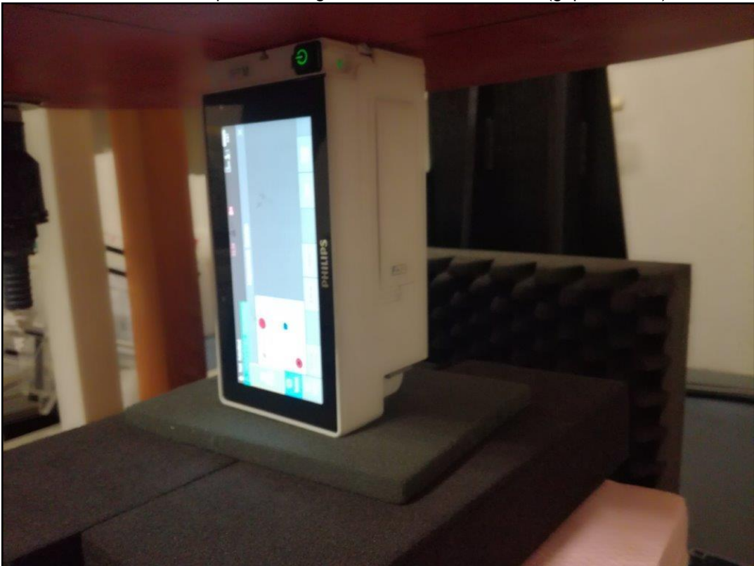
Photo 10: Test position - Right side with 0mm distance (grip removed)
