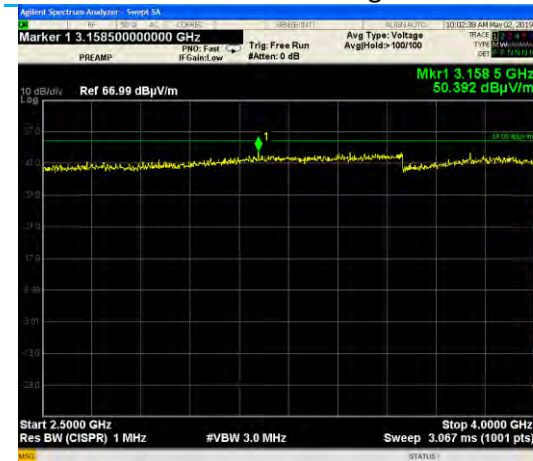
2500-4000 MHz, GFSK, Low Channel, Vertical Antenna, Peak with Average Limit
