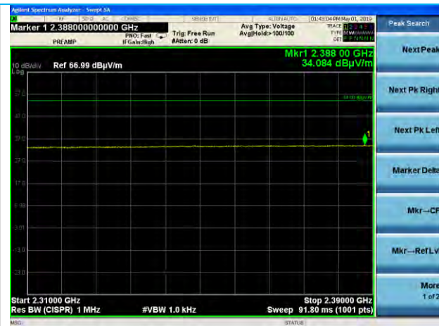
2310-2390 MHz, EUT Flat, EDR2, Low Channel Average
