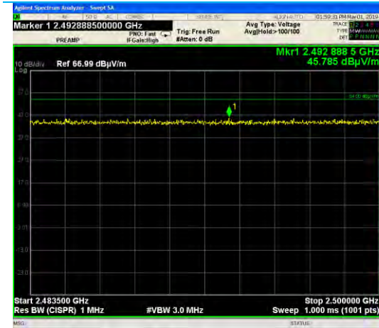
2483.5-2500 MHz, EUT Flat, Hopping Peak with Average Limit
