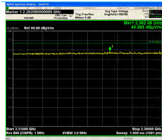
2310-2390 MHz, EUT Flat, EDR2, Low Channel Peak with Average Limit
