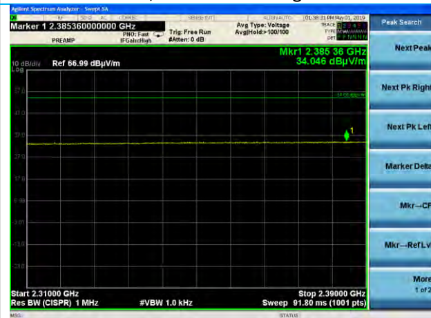
2310-2390 MHz, EUT Flat, GFSK, Low Channel Average
