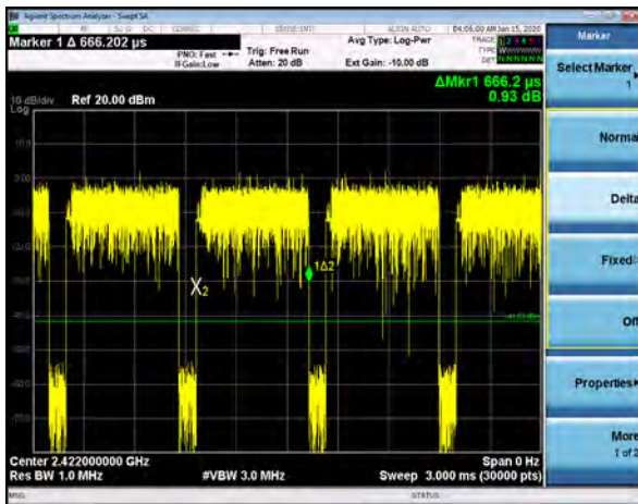
Duty Cycle, 802.11n HT40, MCS0, On Time
