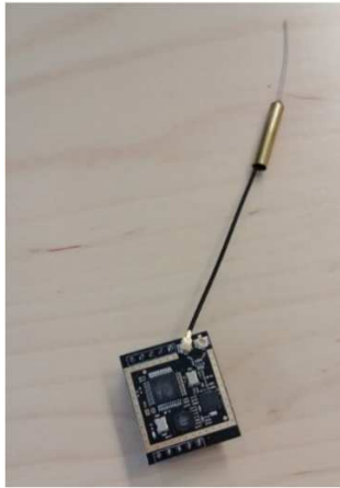
Functional Device: module showing on the left 2.4Ghz frequency hopping GFSK (Device A)
