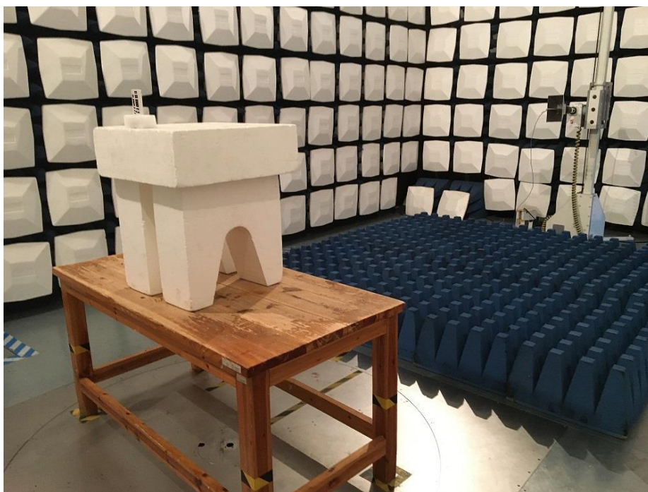
Test Setup For Radiated Emission (Above 1GHz)
