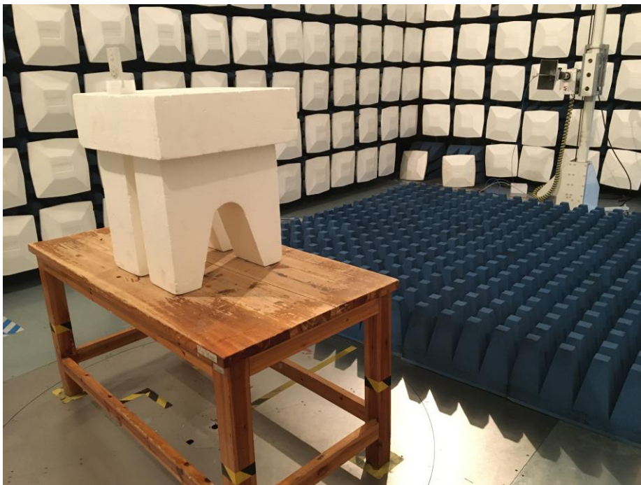
Test Setup For Radiated Emission (Above 1GHz)
