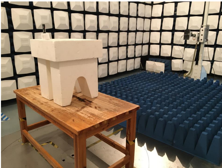
Test Setup For Radiated Emission (Above 1GHz)
