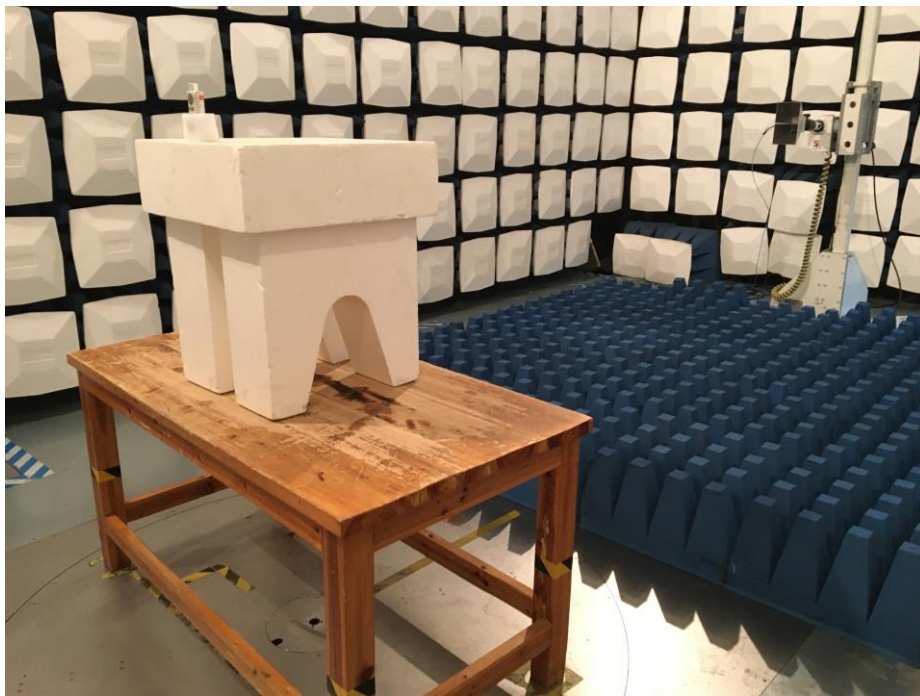
Test Setup For Radiated Emission (Above 1GHz)
