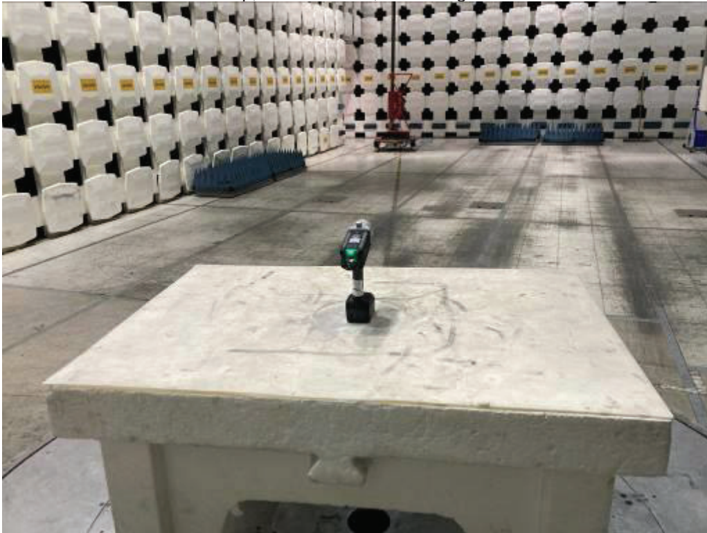
Test Setup, 30-1000 MHz, Pistol Angle Wrench
