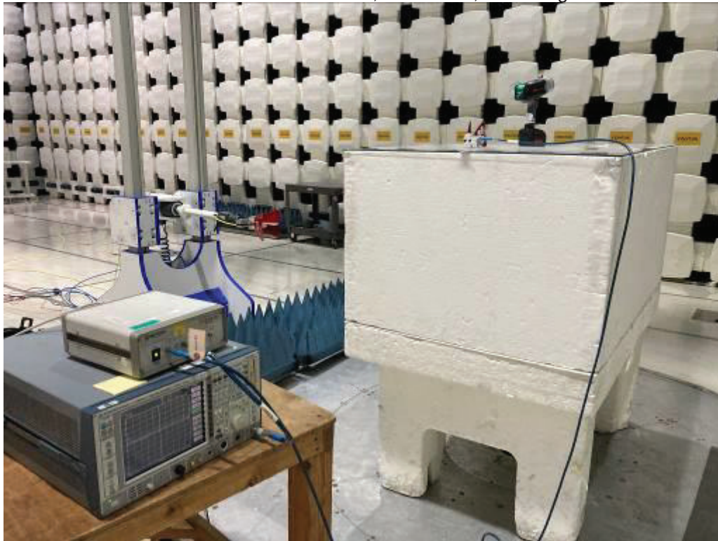
Manual scan at a distance of 10 cm, 18-25 GHz, Pistol Angle Wrench
