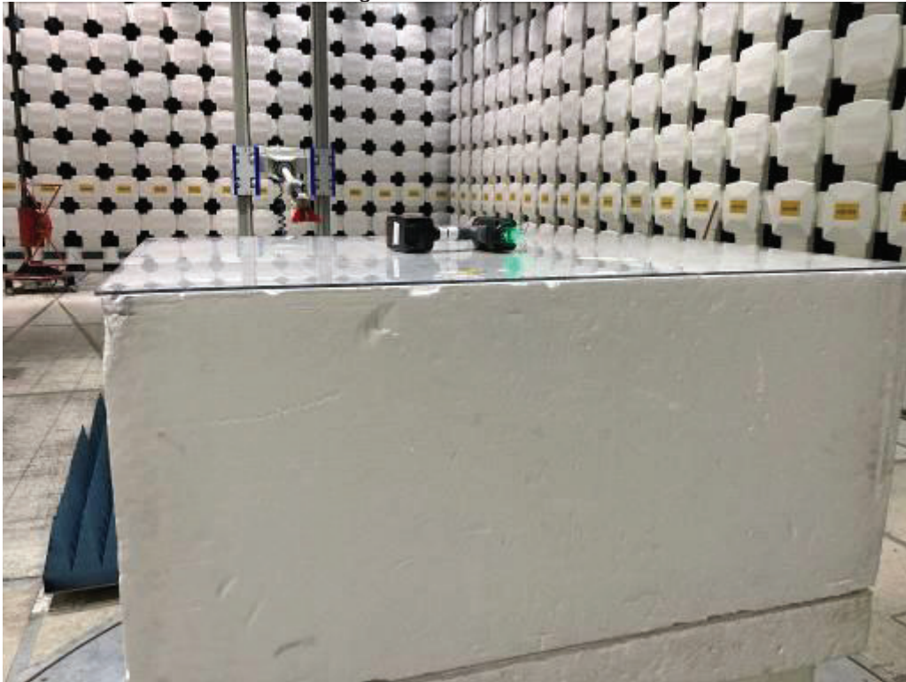
Pistol Angle Wrench, EUT on X-Axis
