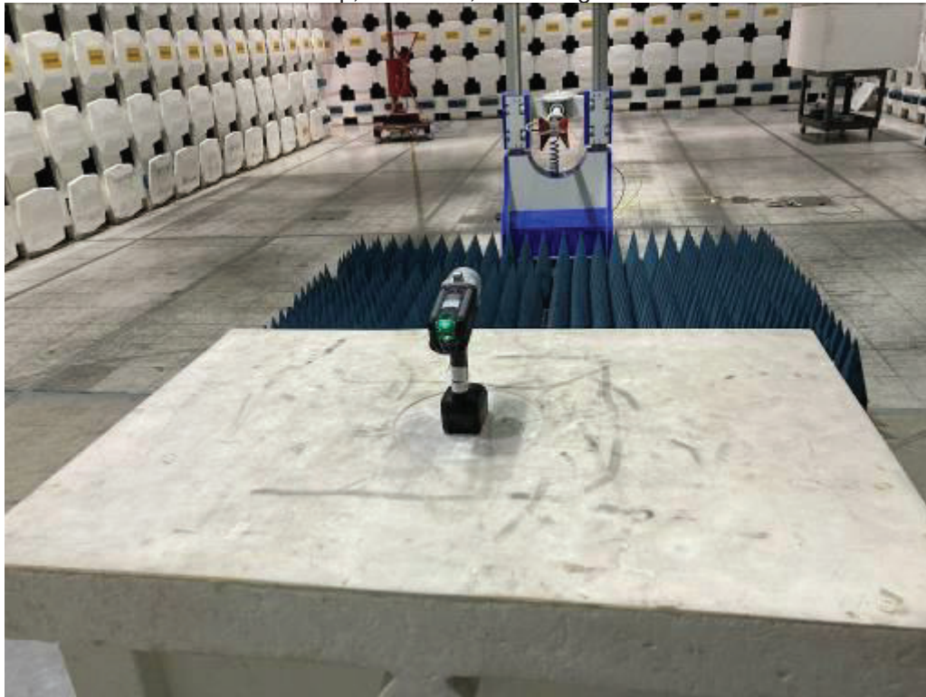
Test Setup, 1-13 GHz, Pistol Angle Wrench
