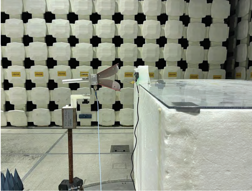
Radiated Emissions Manual Scan Test Setup, 18-25 GHz
