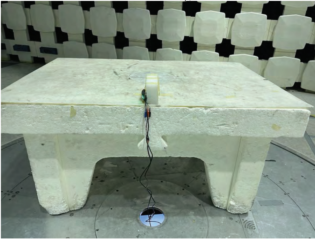
Radiated Emissions Test Setup, 30-1000 MHz
