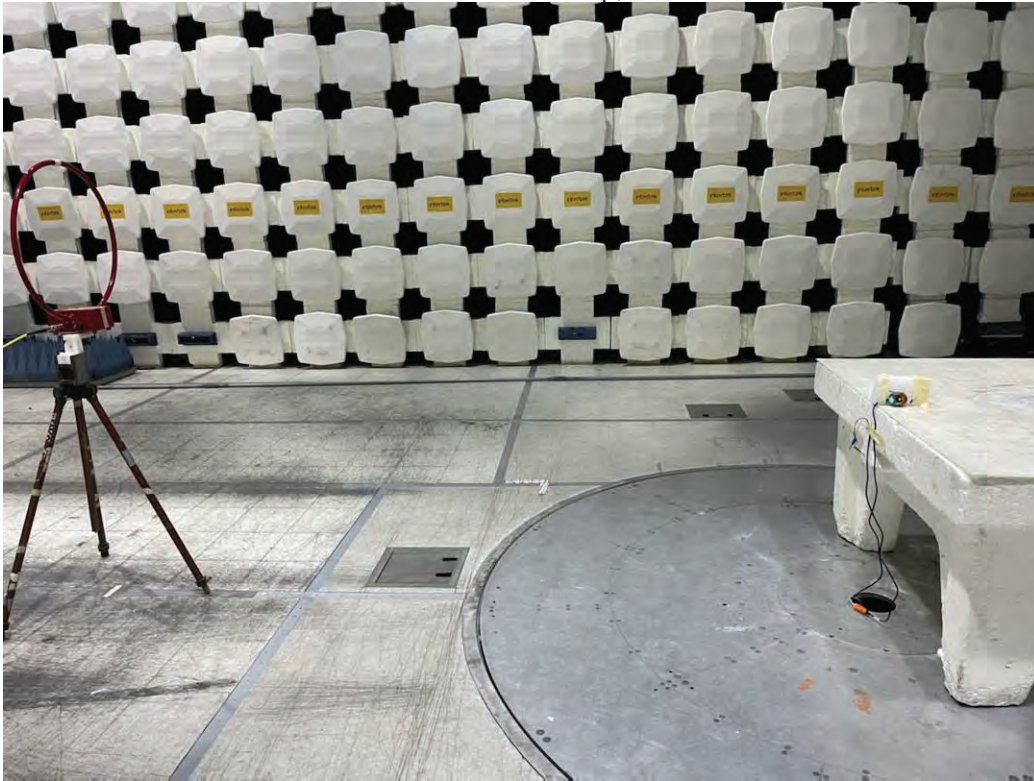
Radiated Emissions Test Setup, 9 kHz-30 MHz
