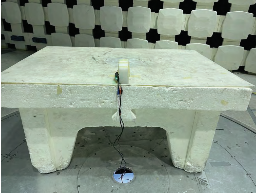
Radiated Emissions Test Setup (Long Side), 30-1000 MHz
