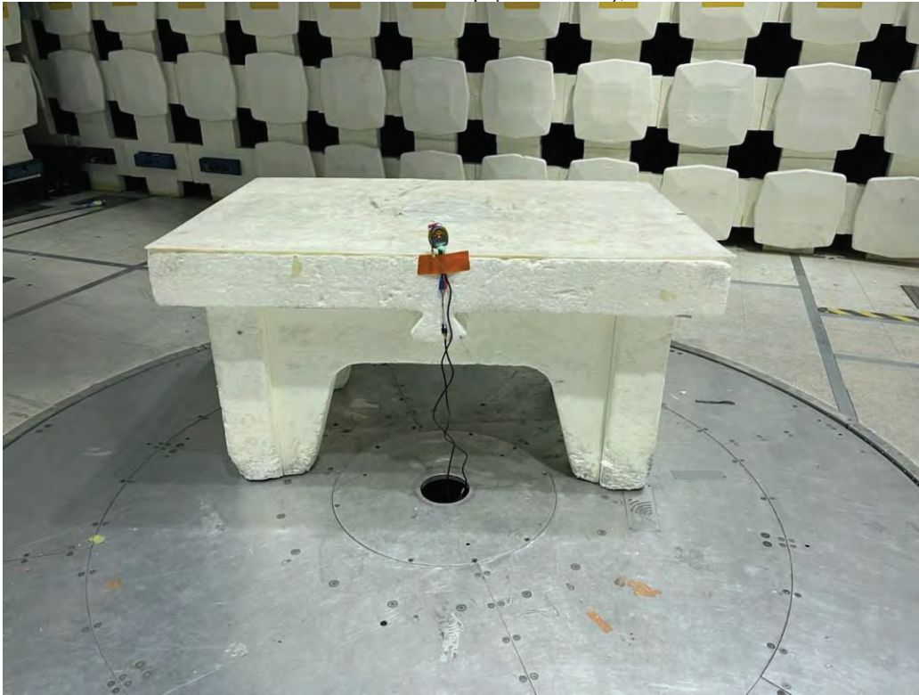
Radiated Emissions Test Setup (Short Side), 30-1000 MHz
