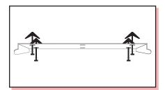
4. Place the bolts with washer through the wall mount and attach the toggles to bolt as shown above.
