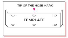
1. On the wall, measure down 7" from the tip of your nose. Place the top of the wall mount level to this point.
