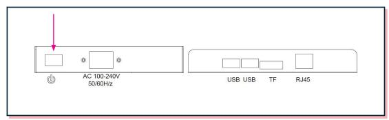
To turn on the Reflect, toggle the power switch into the "ON" position. Then, touch the Echelon® logo on the front. The logo will turn blue when pressed.
