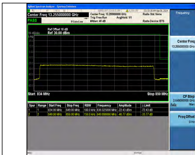
Band26 15MHz 16QAM 26865 1RB#74
