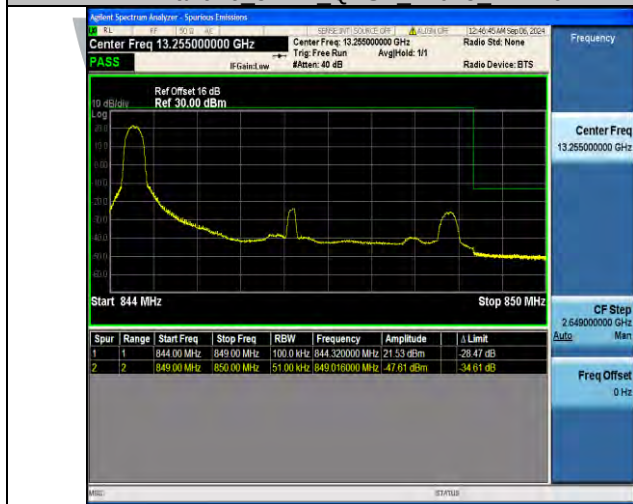
Band26 5MHz QPSK 27015 25RB#0
