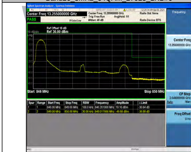
Band26 3MHz 64QAM 27025 15RB#0
