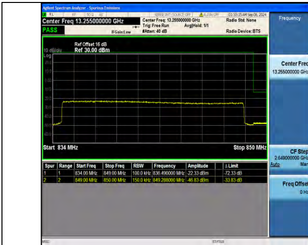
Band38 5MHz QPSK 37775 1RB#24
