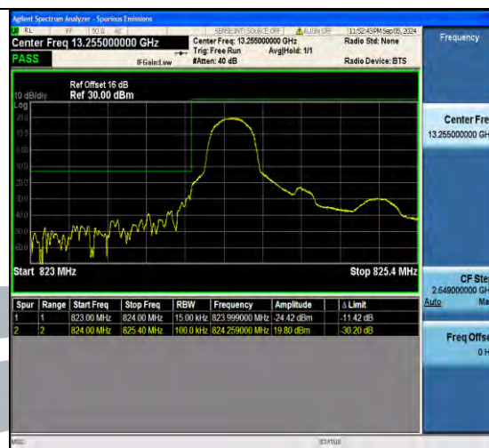
Band26 1.4MHz 64QAM 26797 6RB#0
