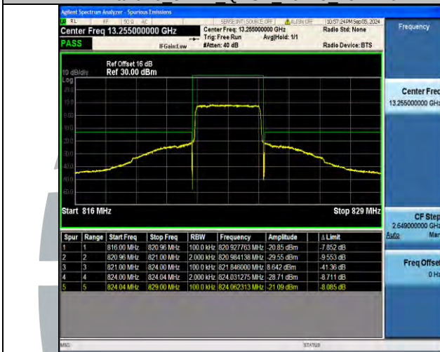
Band26 3MHz 64QAM 26705 1RB#14
