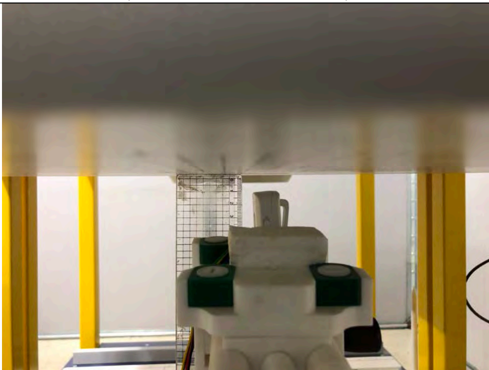
Top of Device 10 mm from Phantom Side view
