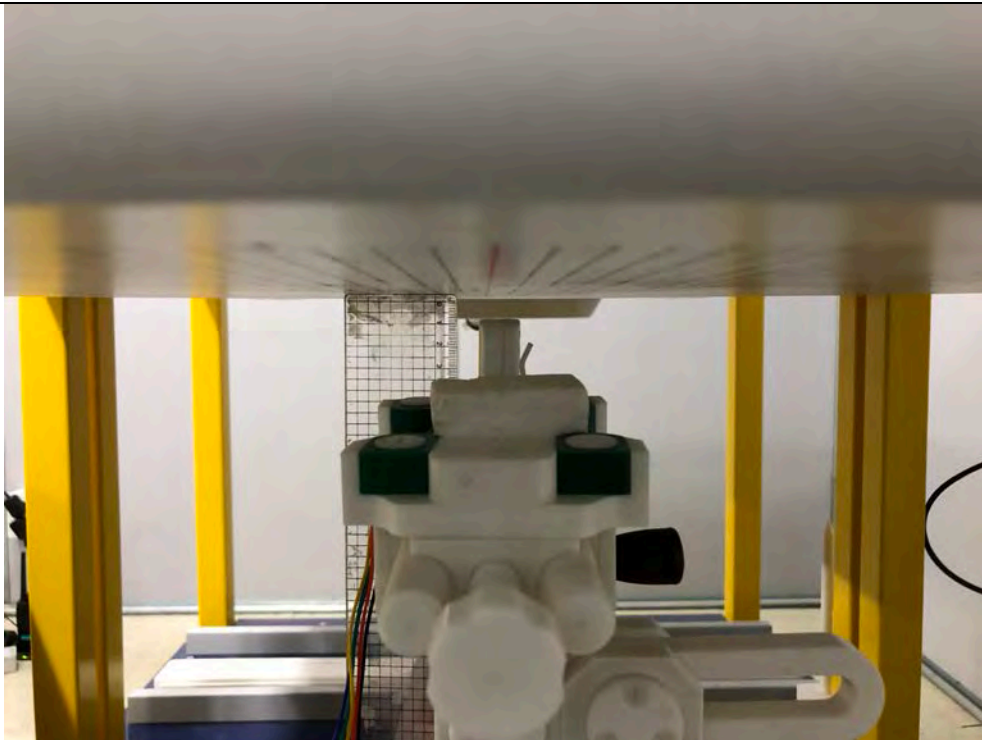
Bottom of Device 10 mm from Phantom Side view
