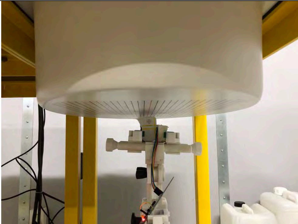
Bottom of Device 10 mm from Phantom Top view
