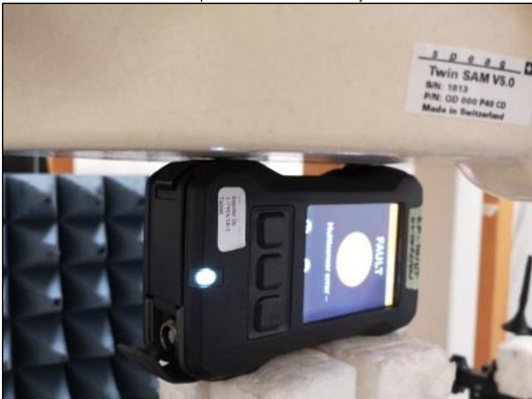
Photo 8: Test position left side without any distance
