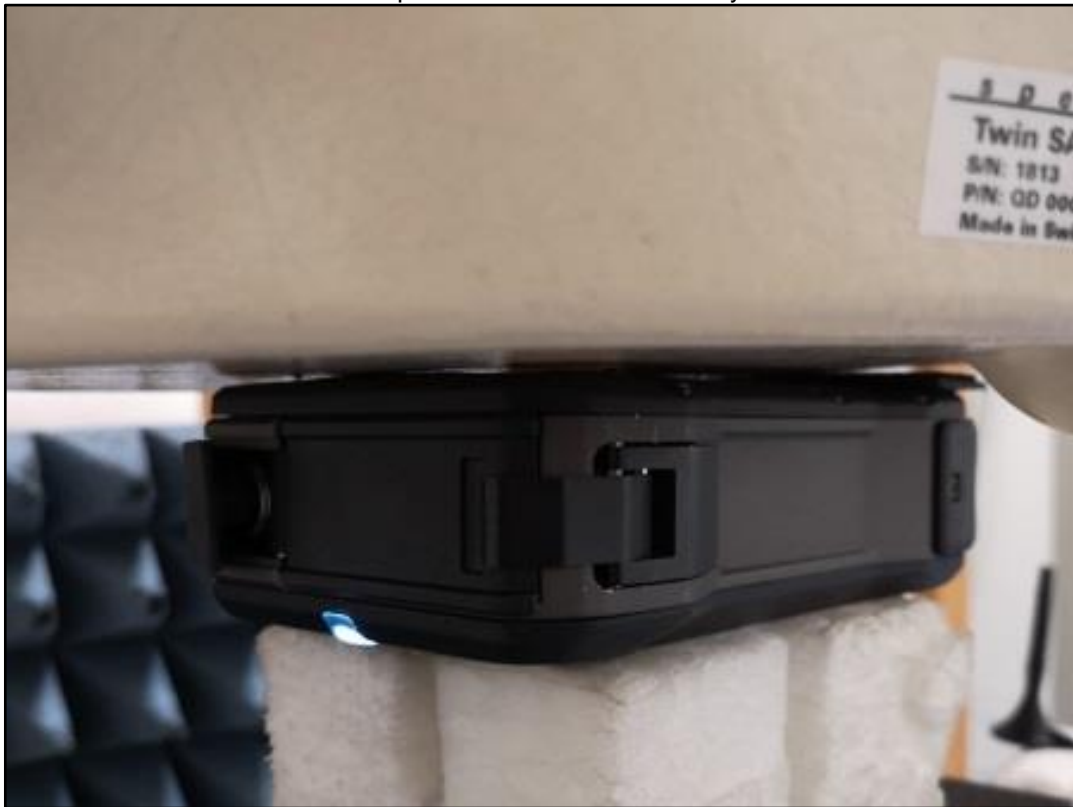
Photo 8: Test position left side without any distance
