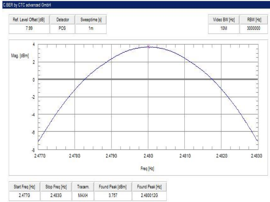
Plot 9: highest channel – 2480 MHz, 8 DPSK modulation
