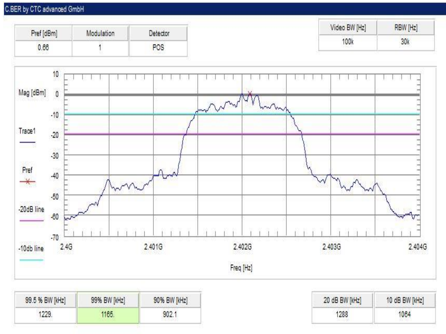
Plot 4: lowest channel – 2402 MHz, Pi / DQPSK modulation
