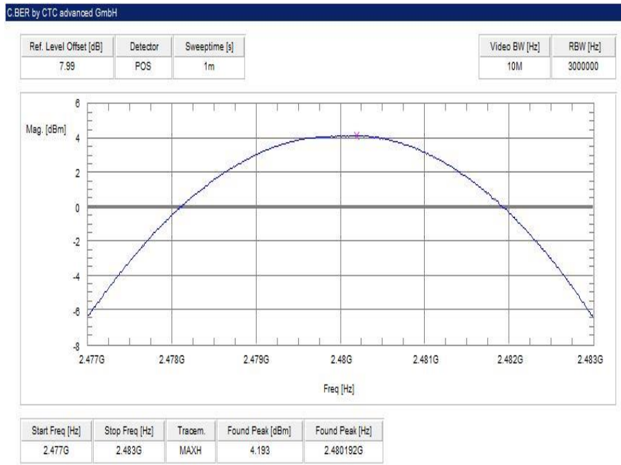
Plot 6: highest channel – 2480 MHz, Pi / DQPSK modulation
