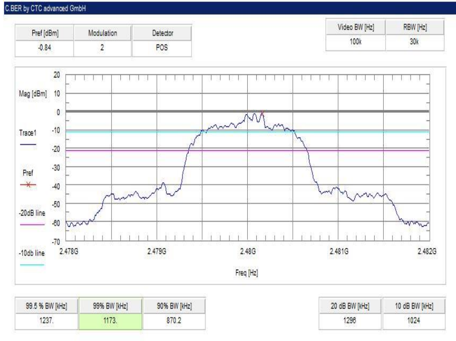
Plot 9: highest channel – 2480 MHz, 8 DPSK modulation
