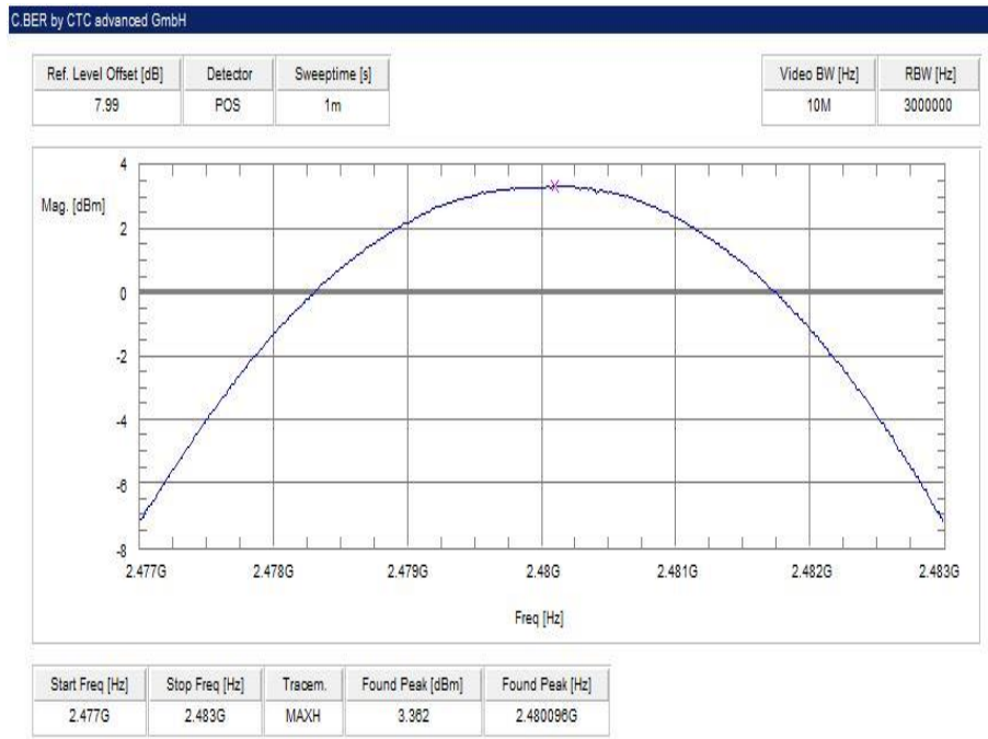
Plot 6: highest channel – 2480 MHz, Pi / DQPSK modulation
