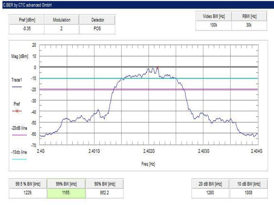
Plot 7: lowest channel – 2402 MHz, 8 DPSK modulation
