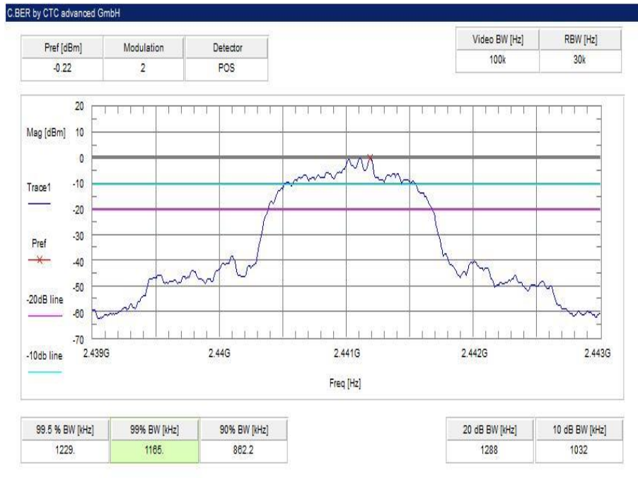
Plot 8: middle channel – 2441 MHz, 8 DPSK modulation
