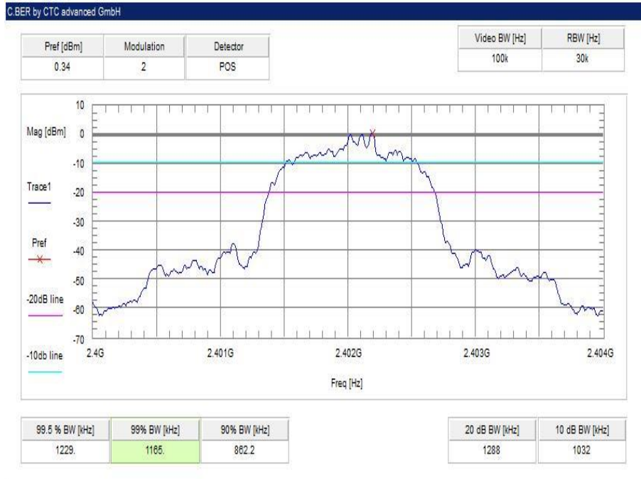
Plot 7: lowest channel – 2402 MHz, 8 DPSK modulation
