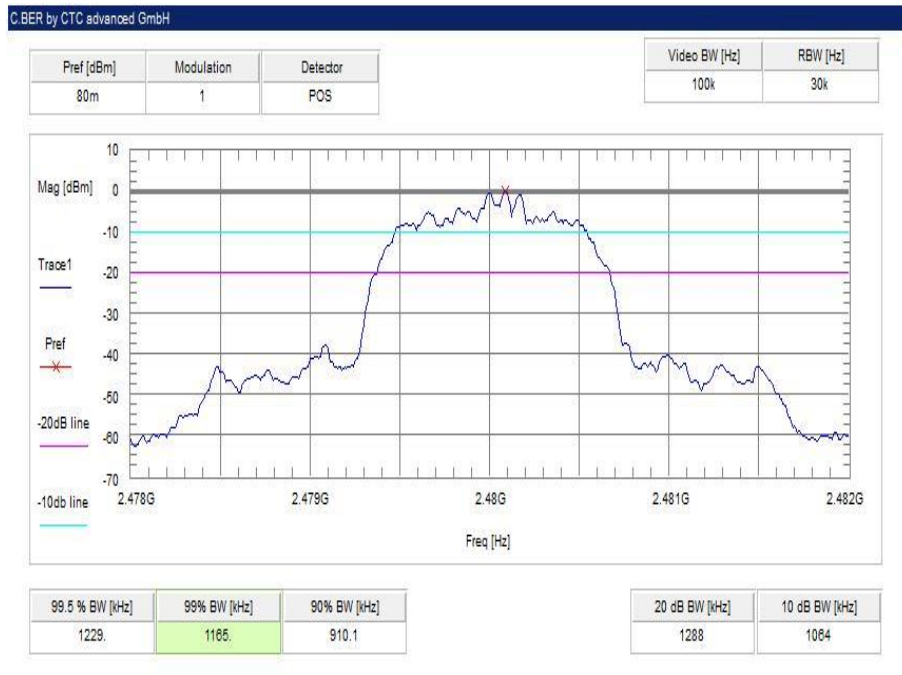
Plot 6: highest channel – 2480 MHz, Pi / DQPSK modulation
