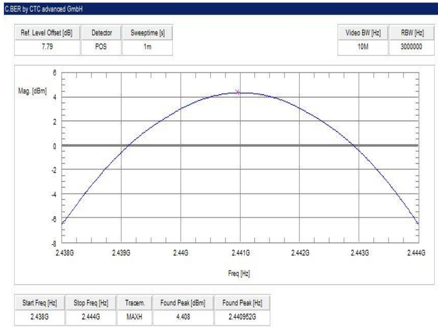
Plot 8: middle channel – 2441 MHz, 8 DPSK modulation
