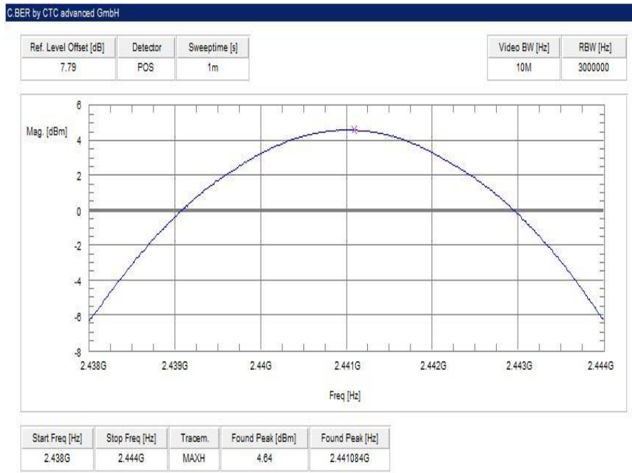
Plot 8: middle channel – 2441 MHz, 8 DPSK modulation
