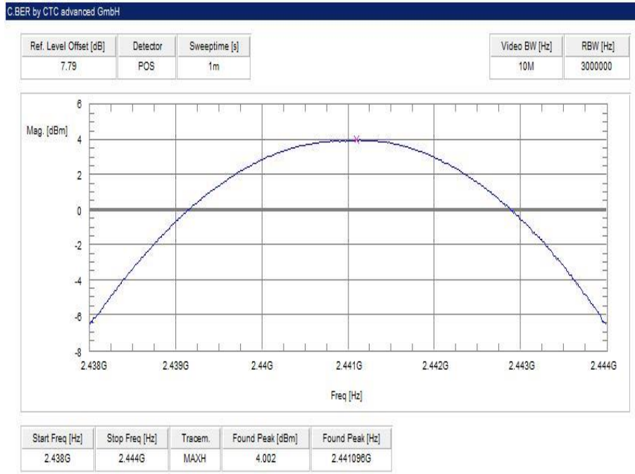
Plot 5: middle channel – 2441 MHz, Pi / DQPSK modulation
