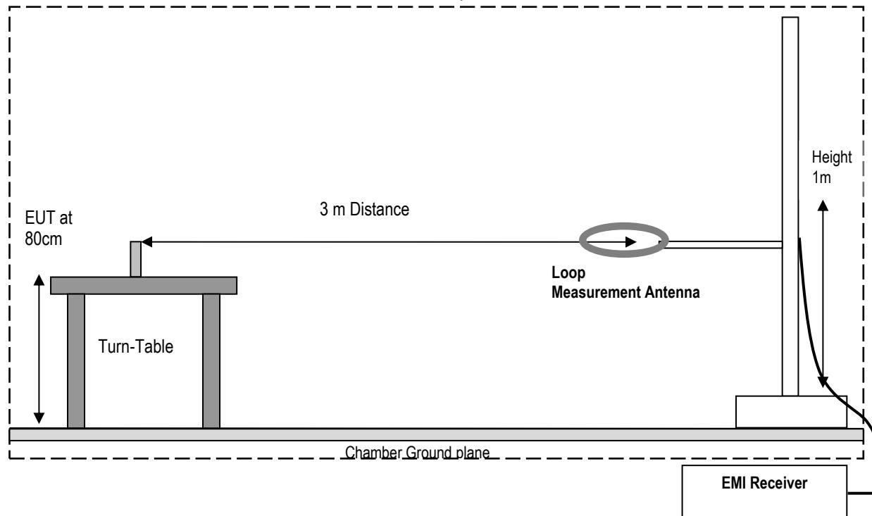
Radiated Emissions Test Setup 30MHz-1GHz Measurements
