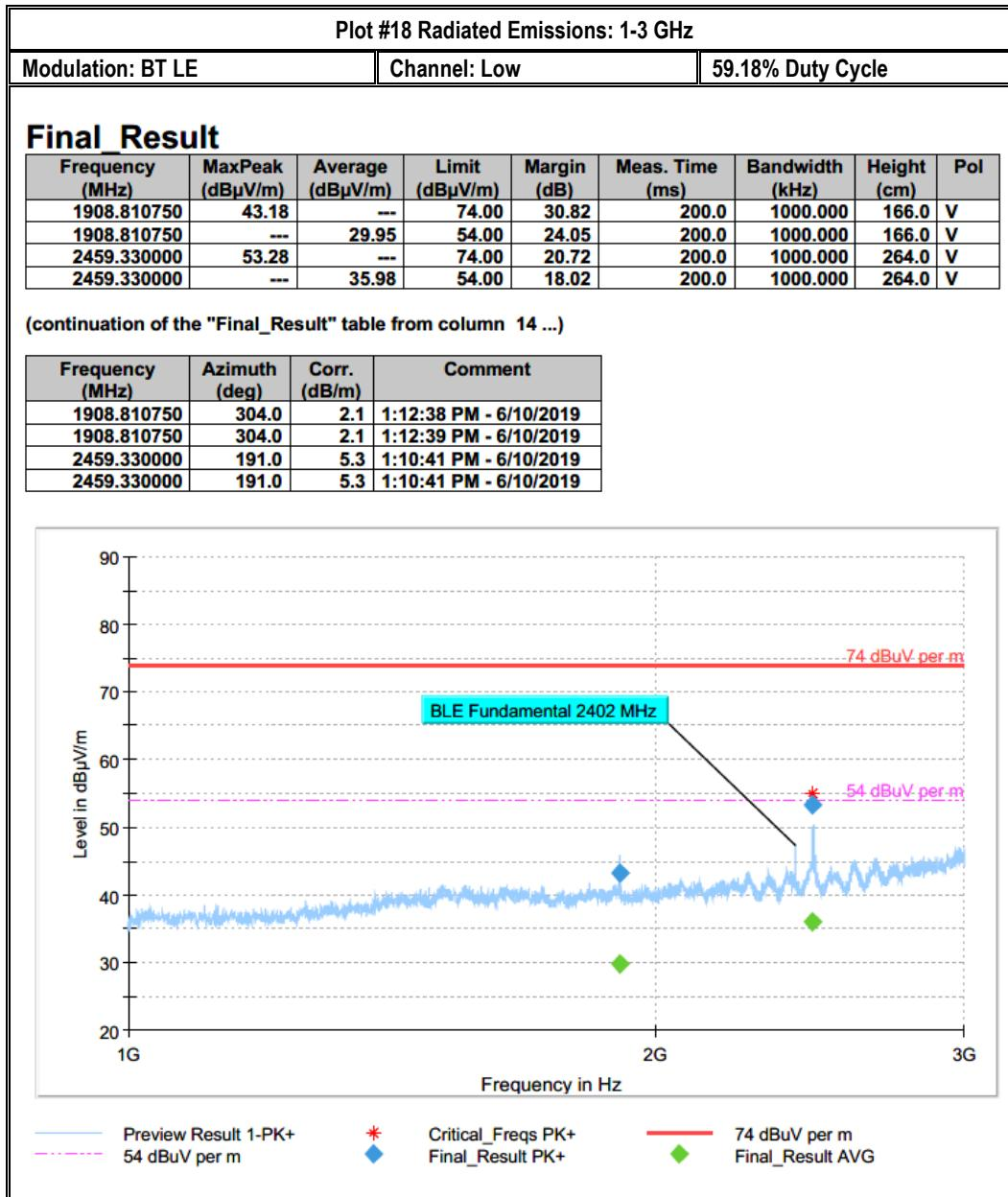
**Note:** Notch filter utilized to attenuate fundamental signal
