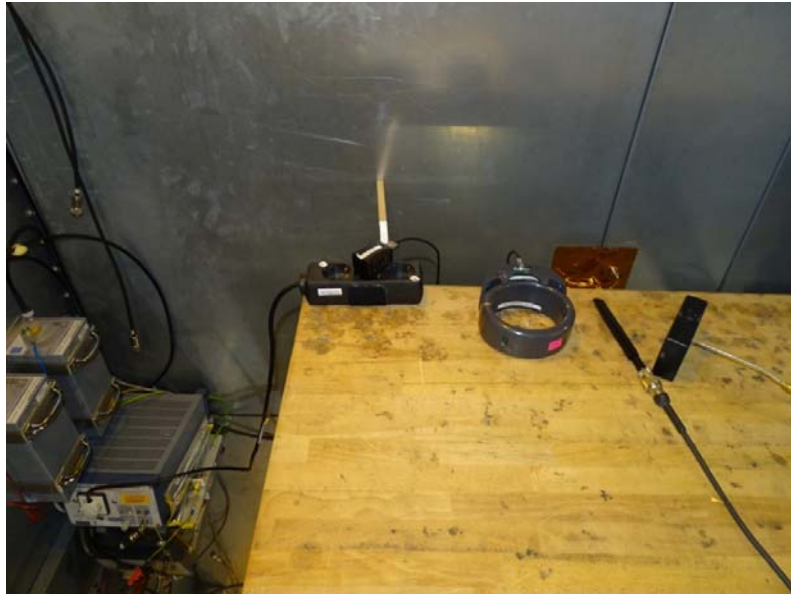
Photo 1: Test setup for conducted emissions (AC Power Line)
