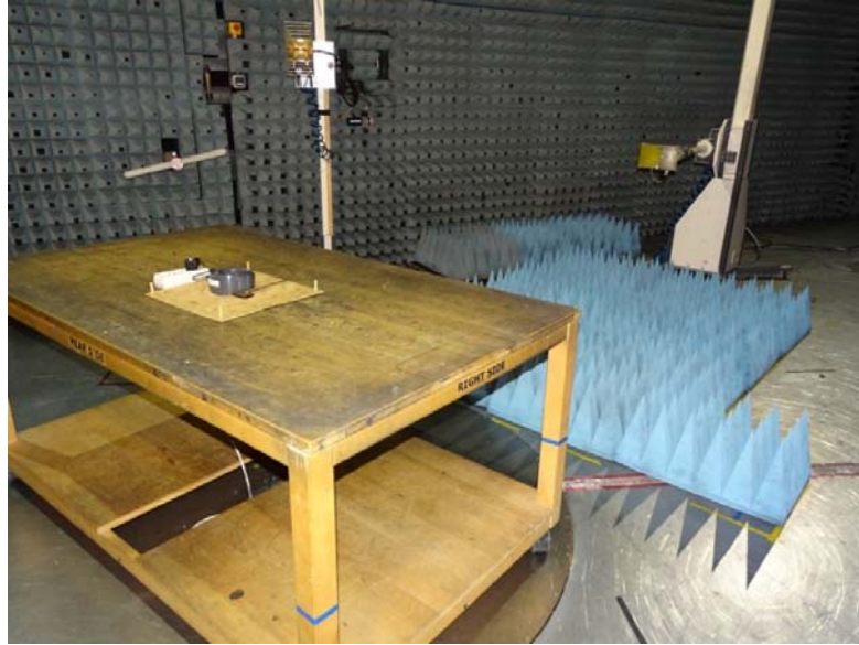
Photo 3: Test setup for radiated measurements above 1 GHz
