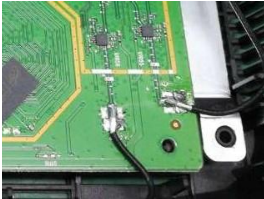
The 2.4GHz WiFi antenna is not removable
