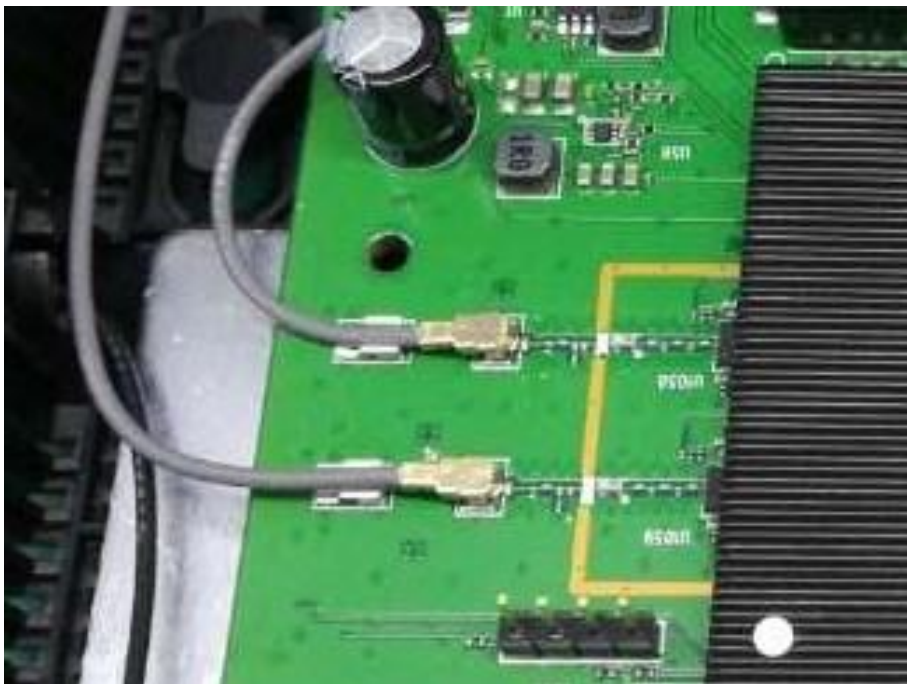
The 5GHz WiFi antenna is revised SMA connector
