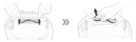
**Set roller brush assembly:** take out sucking assembly first, set the roller brush and cover the board and then press to lock.
