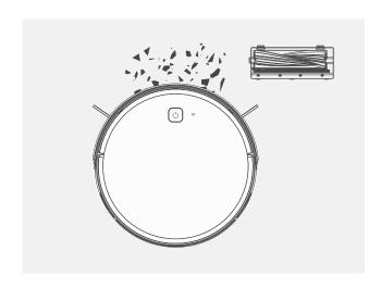
**Set sucking parts:** take Aout roller brush cover board and brush first, and change suction cover board and then press to lock.
