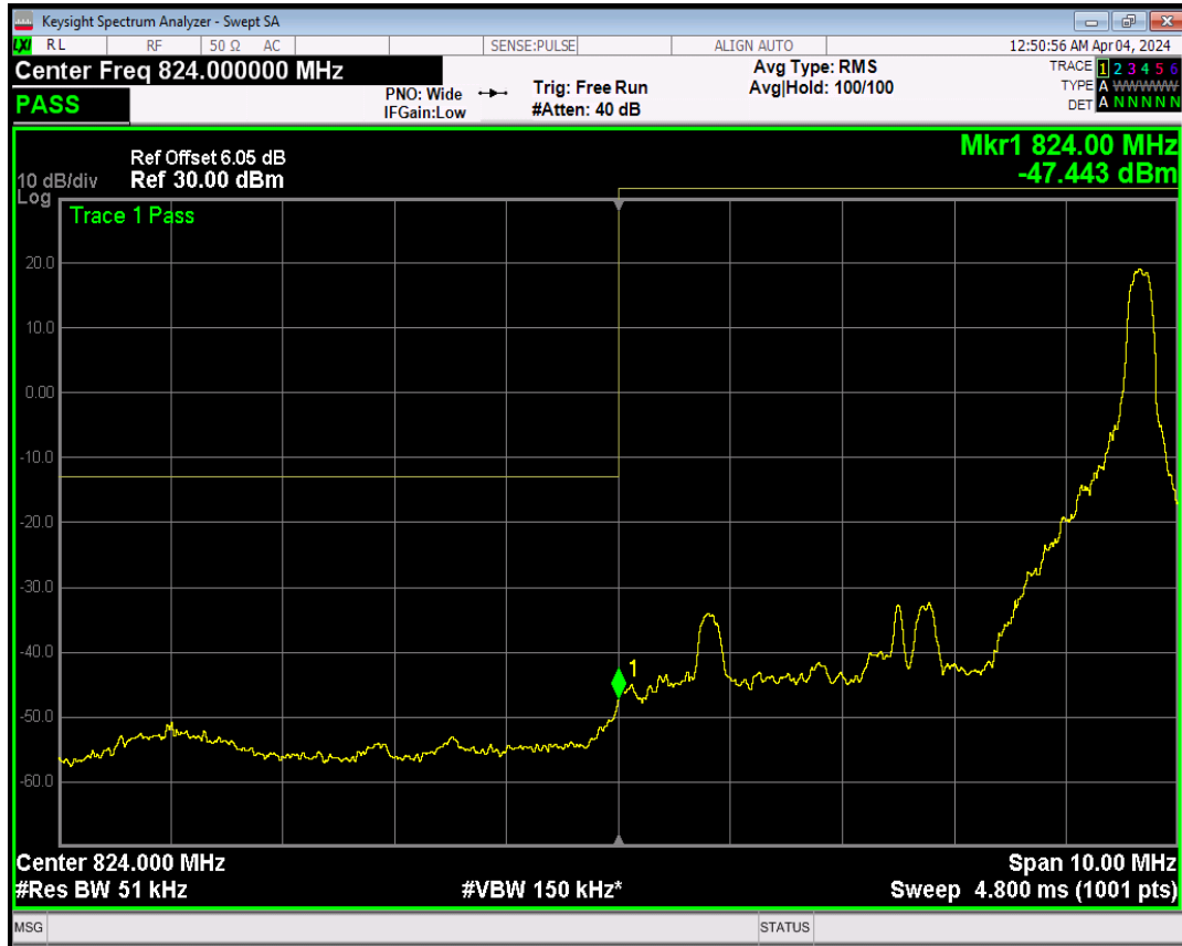
Band5 QPSK BW=5MHz Channel=20425 RB Size=25 Position=#0
