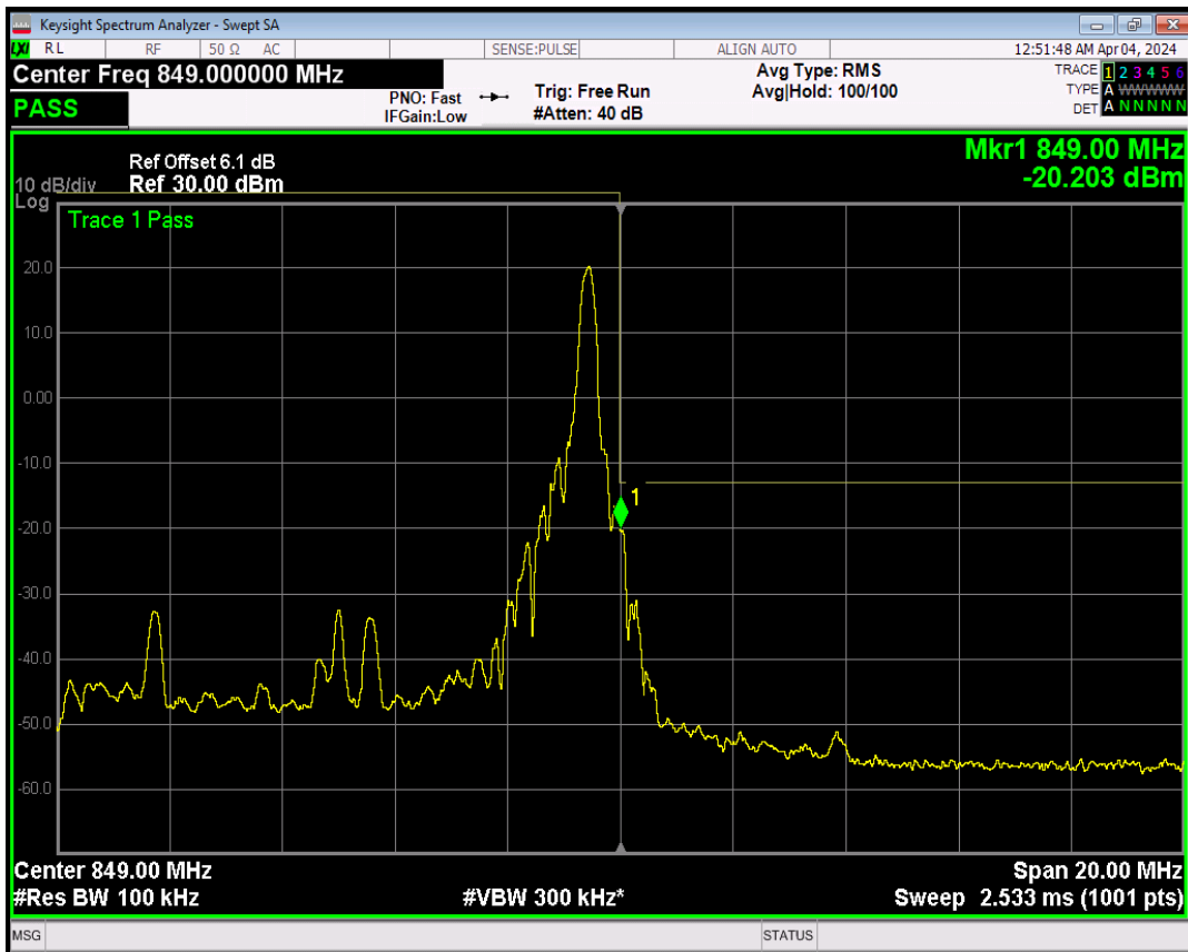
Band5 16QAM BW=10MHz Channel=20600 RB Size=50 Position=#0
