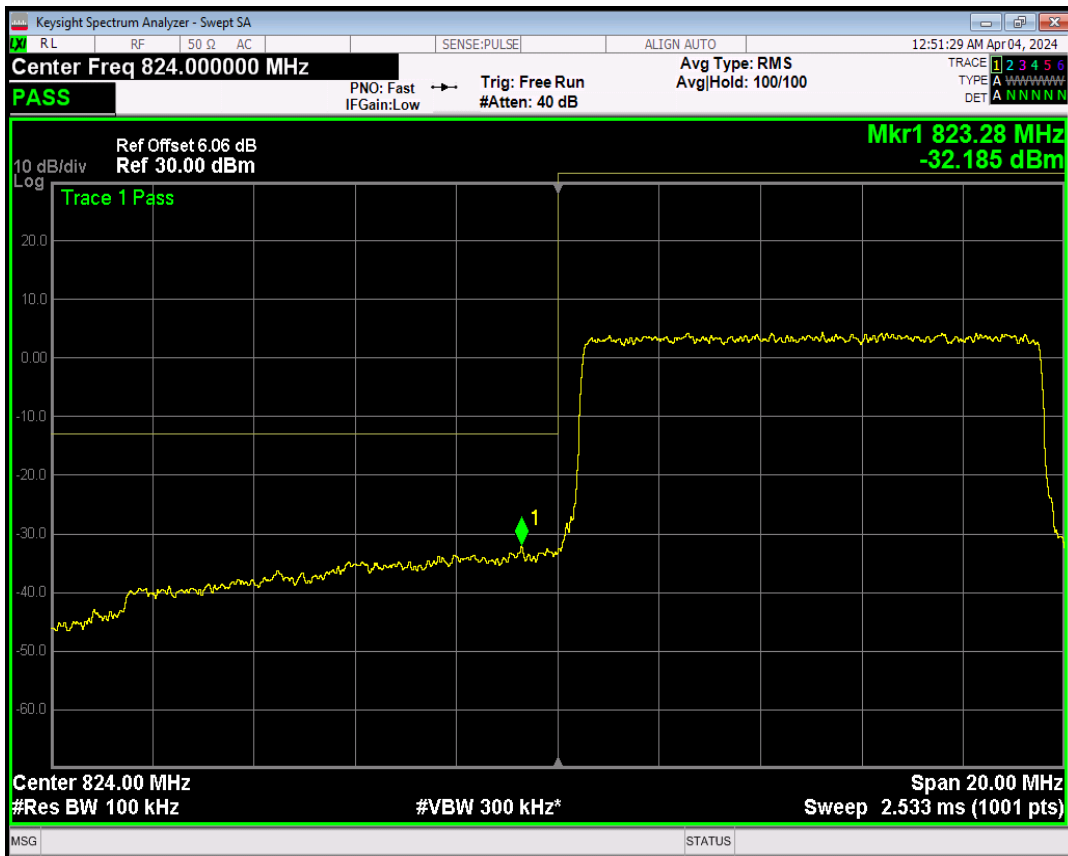
Band5 16QAM BW=10MHz Channel=20450 RB Size=1 Position=#0
