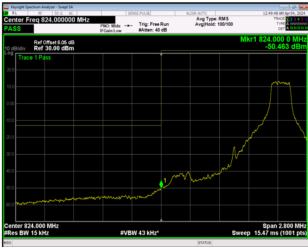
Band5 16QAM BW=1.4MHz Channel=20407 RB Size=6 Position=#0
