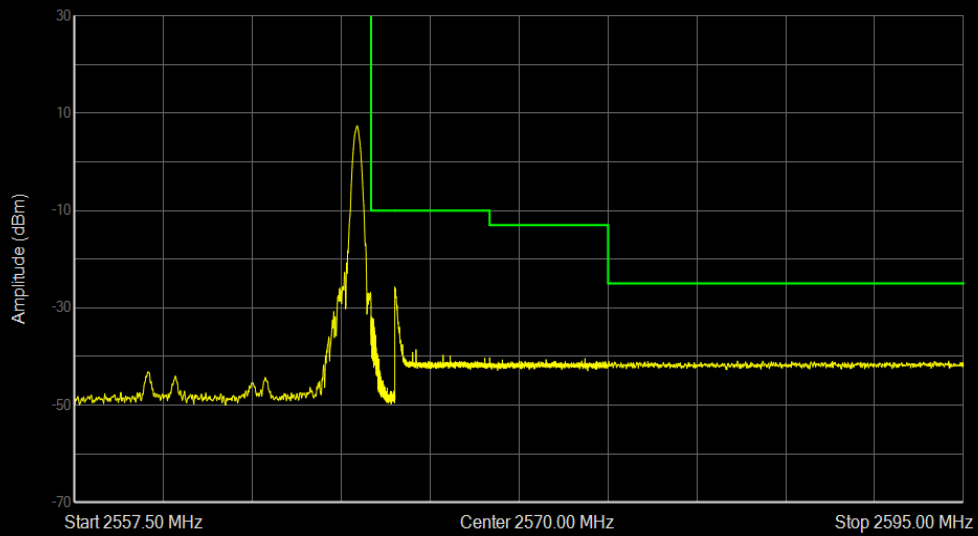
Band7 16QAM BW=10MHz Channel=21400 RB Size=1 Position=#Max
