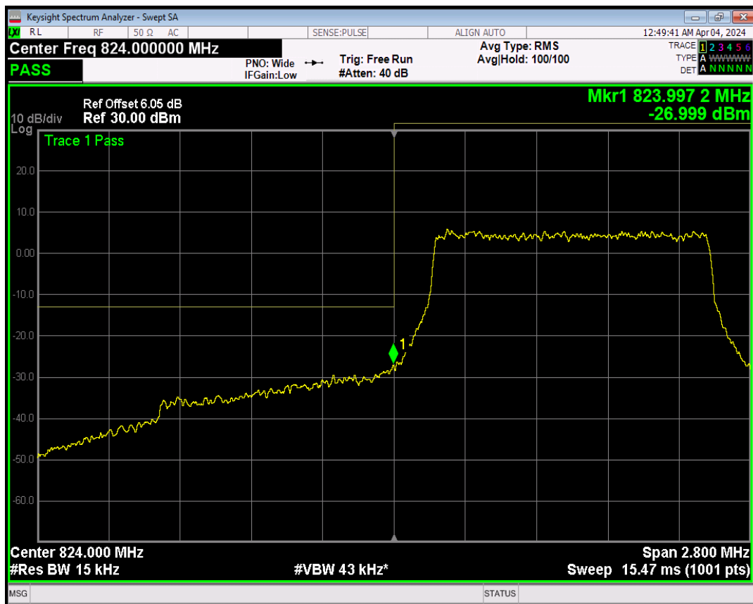
Band5 16QAM BW=1.4MHz Channel=20407 RB Size=1 Position=#0
