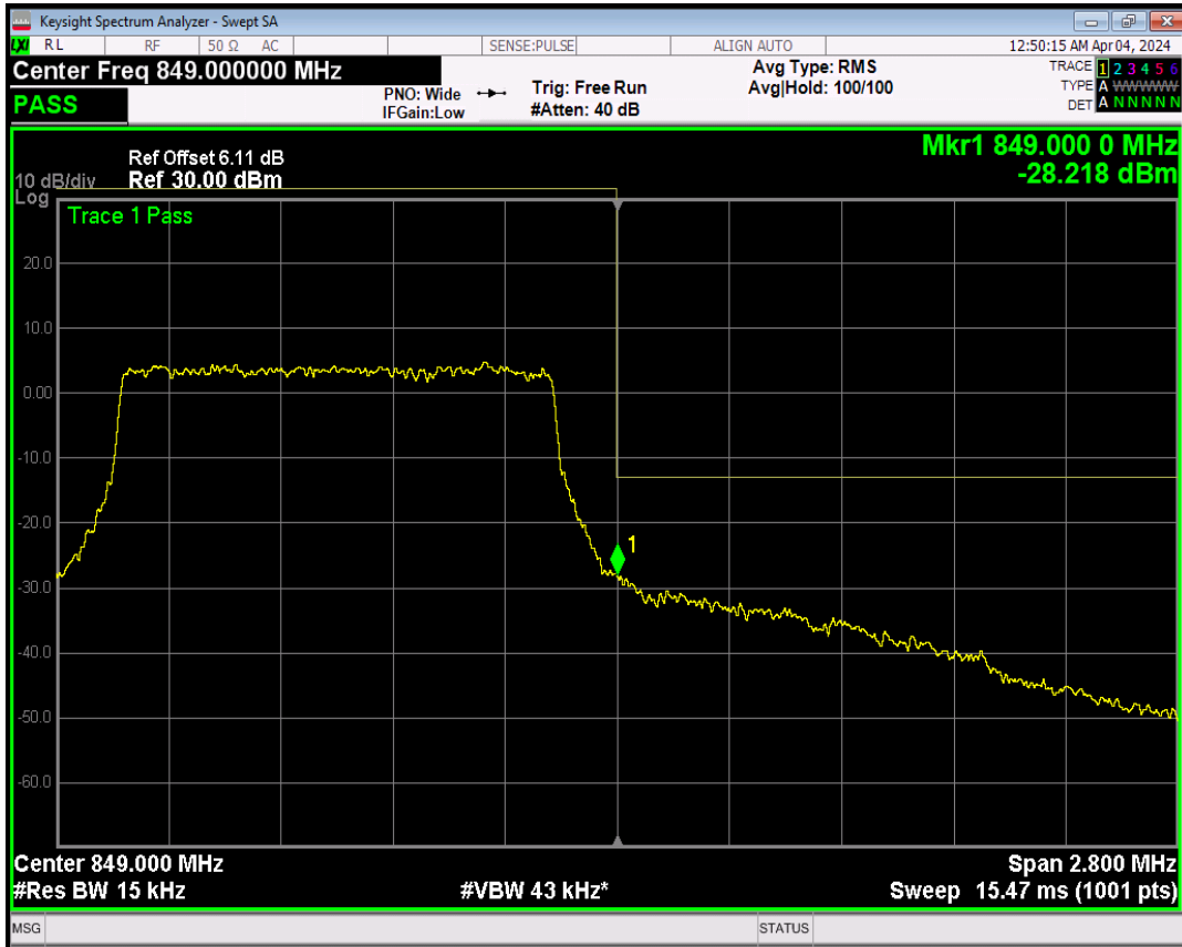
Band5 QPSK BW=3MHz Channel=20415 RB Size=1 Position=#0
