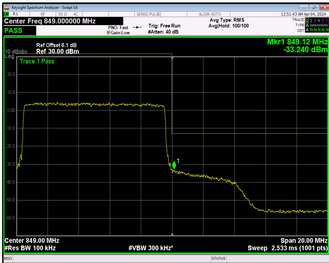
Band5 16QAM BW=10MHz Channel=20600 RB Size=1 Position=#0
