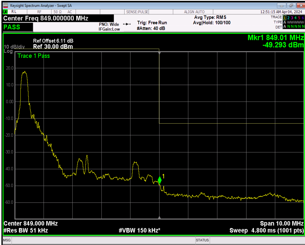
Band5 16QAM BW=5MHz Channel=20625 RB Size=1 Position=#Max
