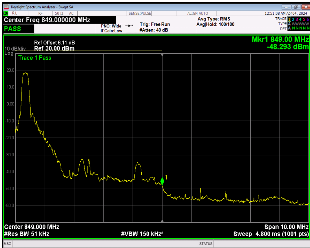
Band5 QPSK BW=5MHz Channel=20625 RB Size=1 Position=#Max
