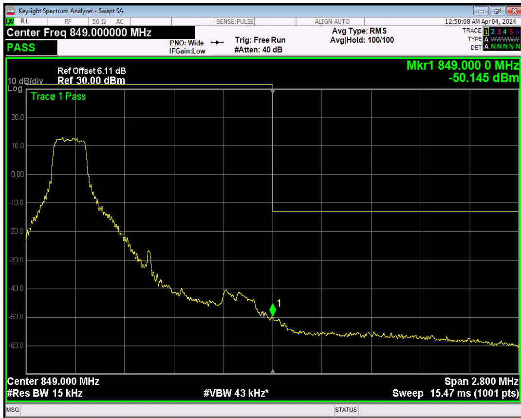
Band5 16QAM BW=1.4MHz Channel=20643 RB Size=1 Position=#Max
