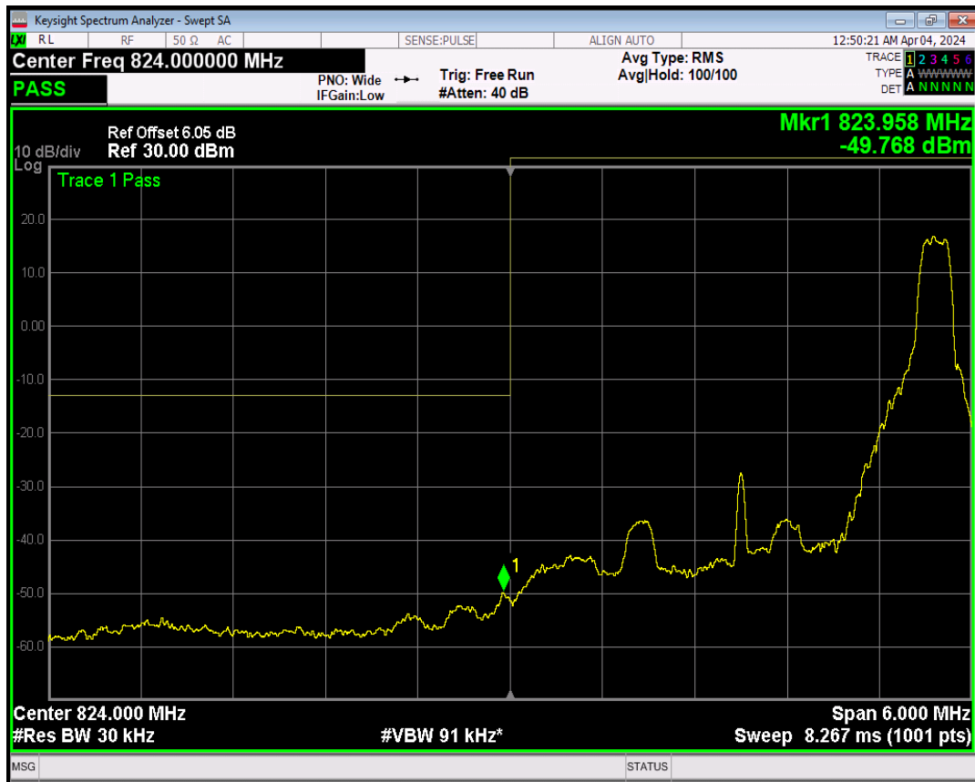
Band5 QPSK BW=3MHz Channel=20415 RB Size=15 Position=#0
