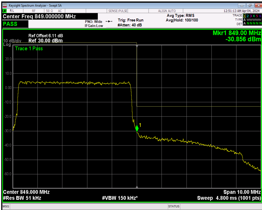
Band5 16QAM BW=5MHz Channel=20625 RB Size=1 Position=#0
