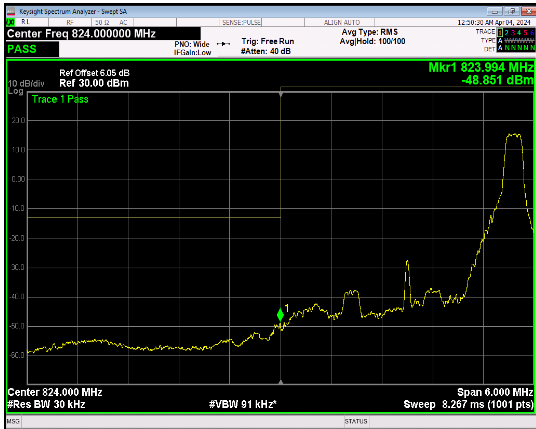
Band5 16QAM BW=3MHz Channel=20415 RB Size=15 Position=#0
