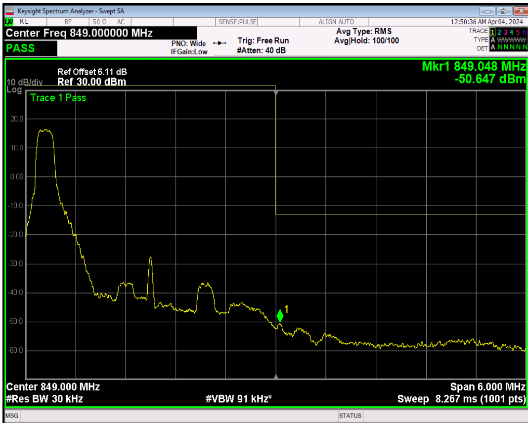
Band5 QPSK BW=3MHz Channel=20635 RB Size=1 Position=#Max
