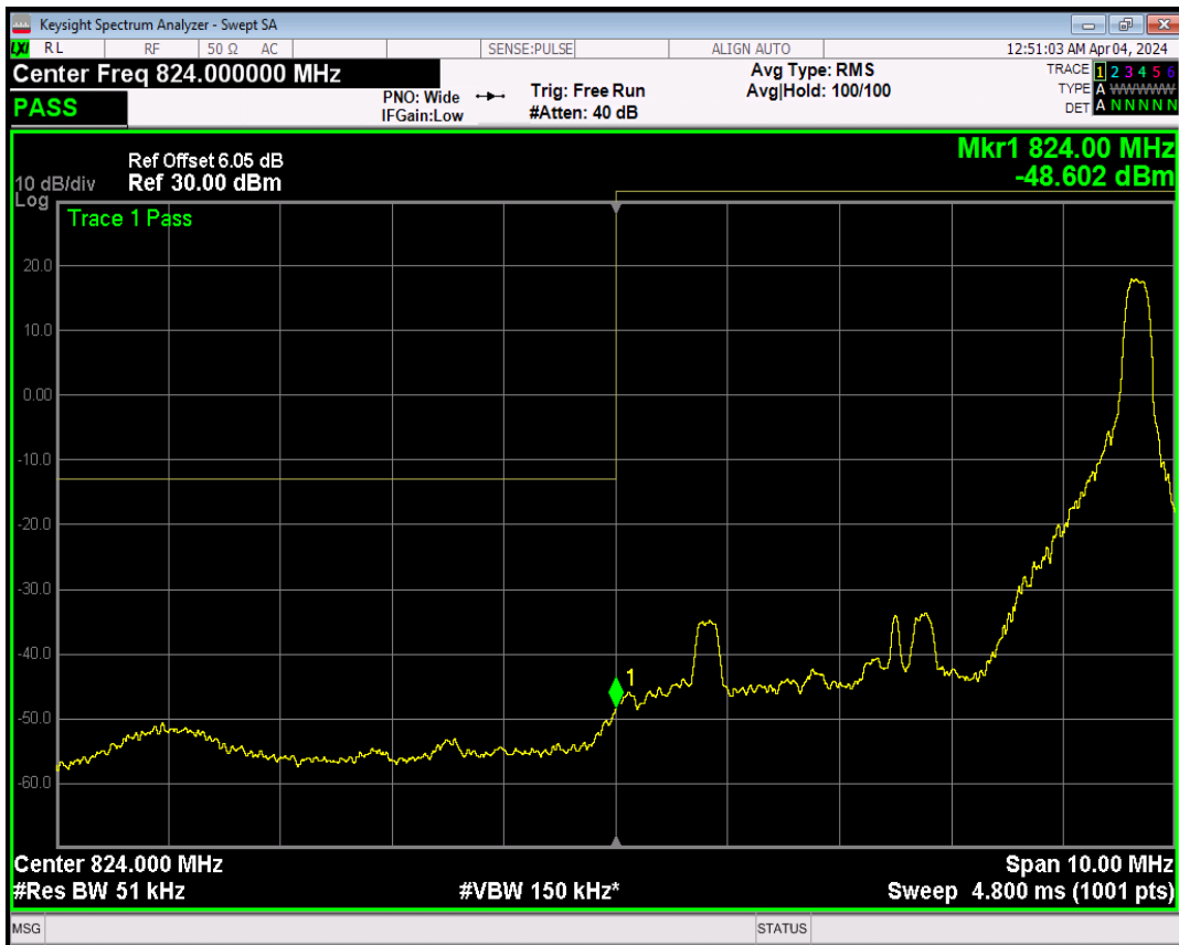
Band5 16QAM BW=5MHz Channel=20425 RB Size=25 Position=#0
