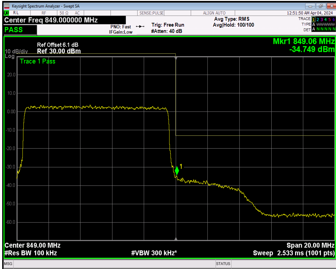
Band7 QPSK BW=5MHz Channel=20775 RB Size=1 Position=#0
