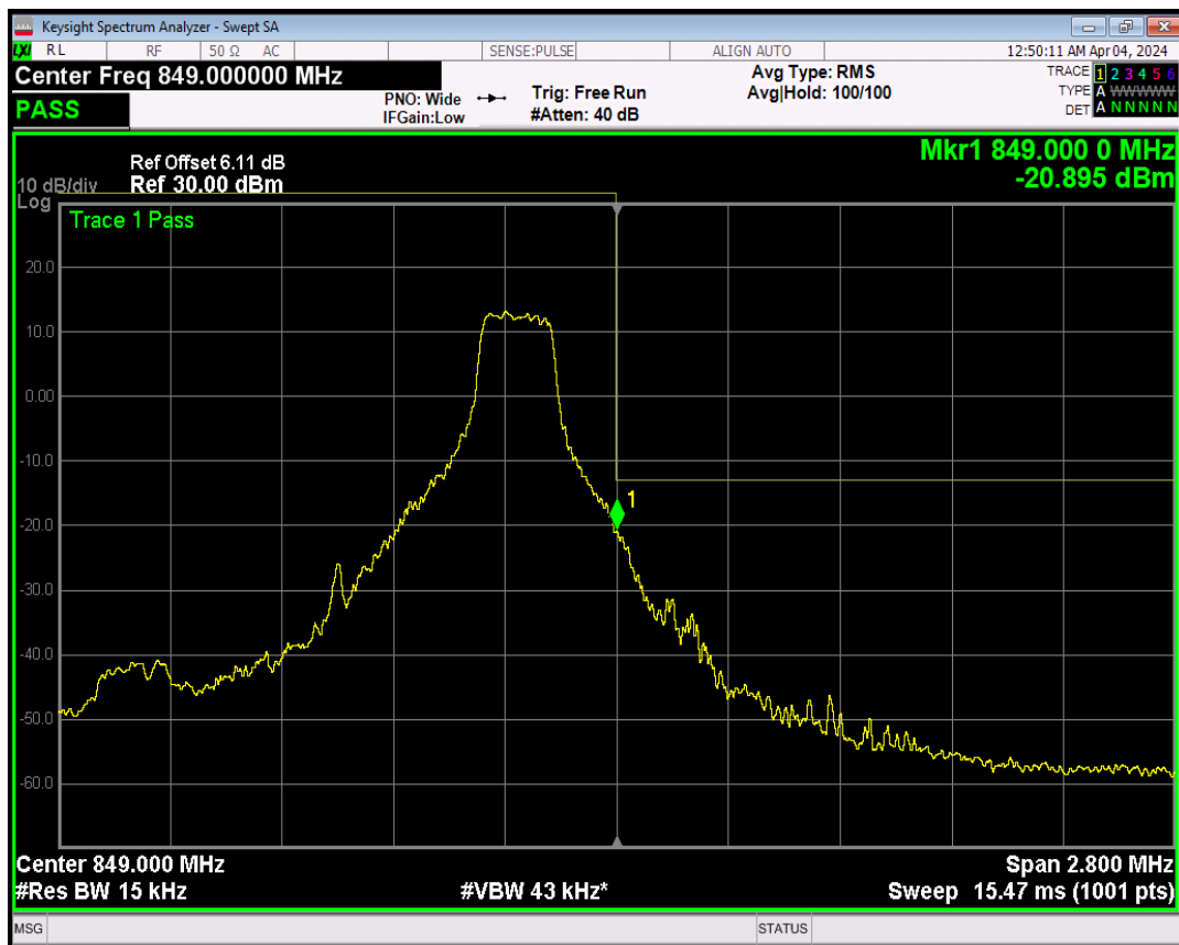
Band5 16QAM BW=1.4MHz Channel=20643 RB Size=6 Position=#0
