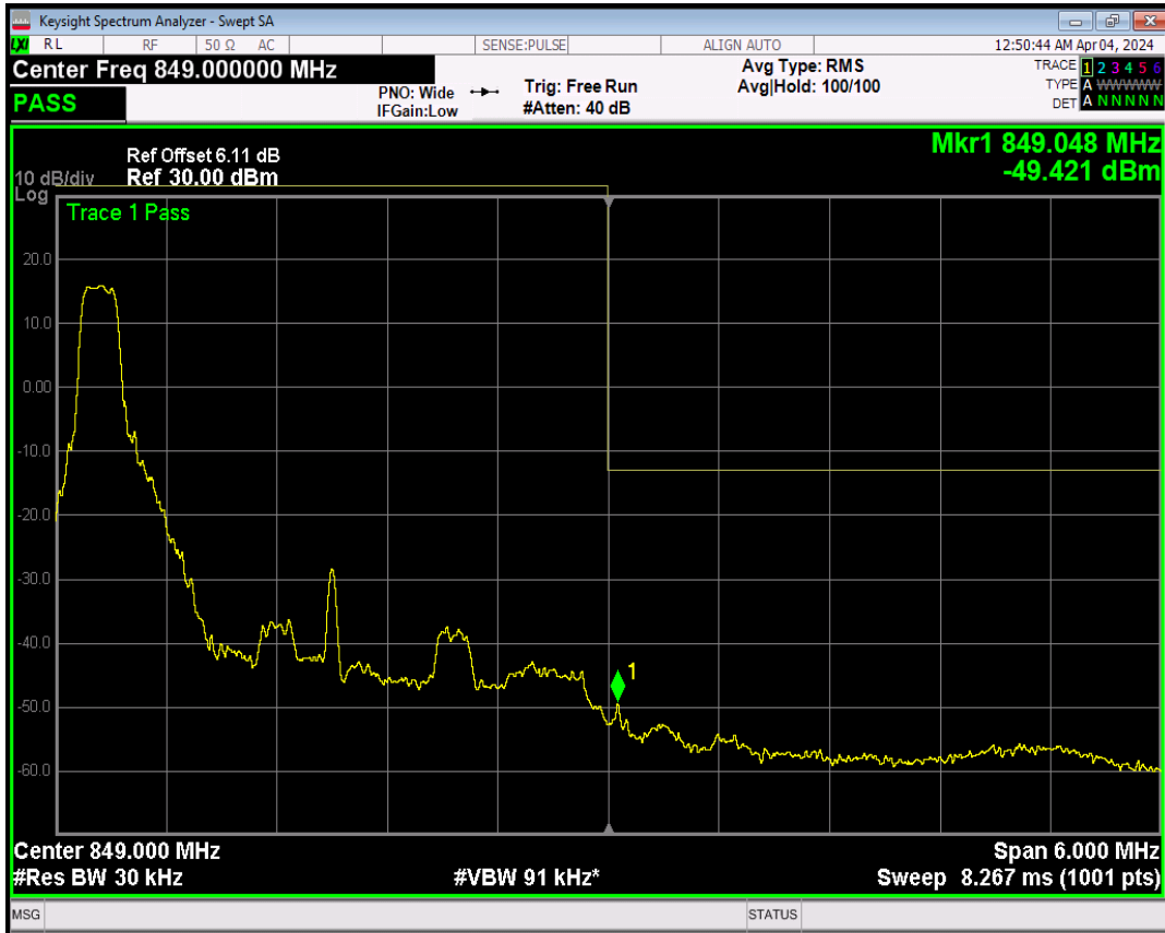
Band5 16QAM BW=3MHz Channel=20635 RB Size=1 Position=#Max
