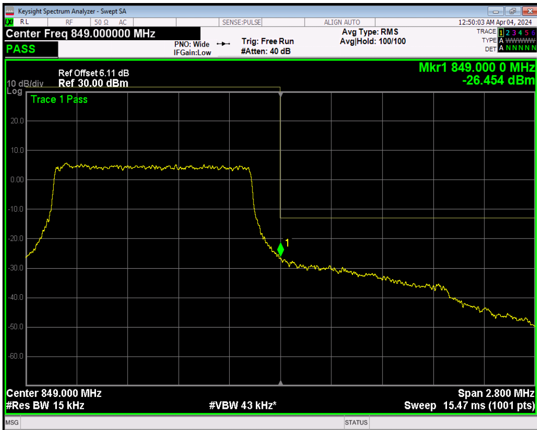
Band5 16QAM BW=1.4MHz Channel=20643 RB Size=1 Position=#0
