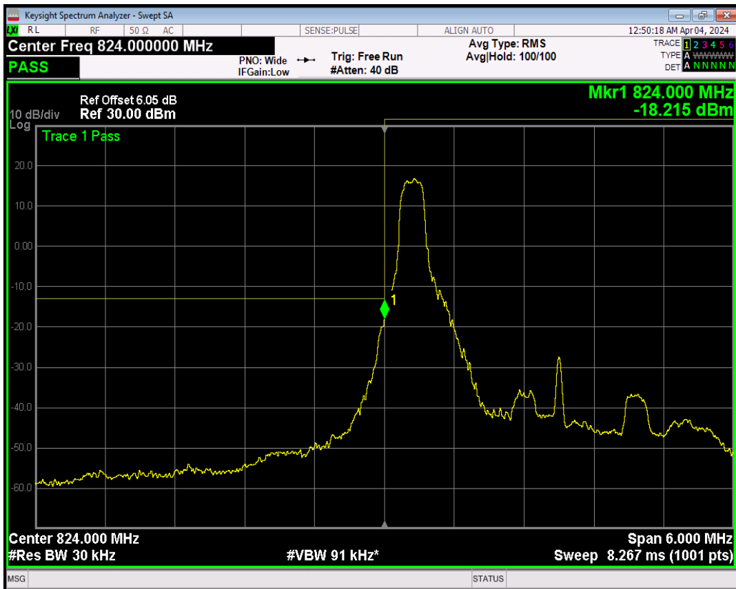
Band5 QPSK BW=3MHz Channel=20415 RB Size=1 Position=#Max
