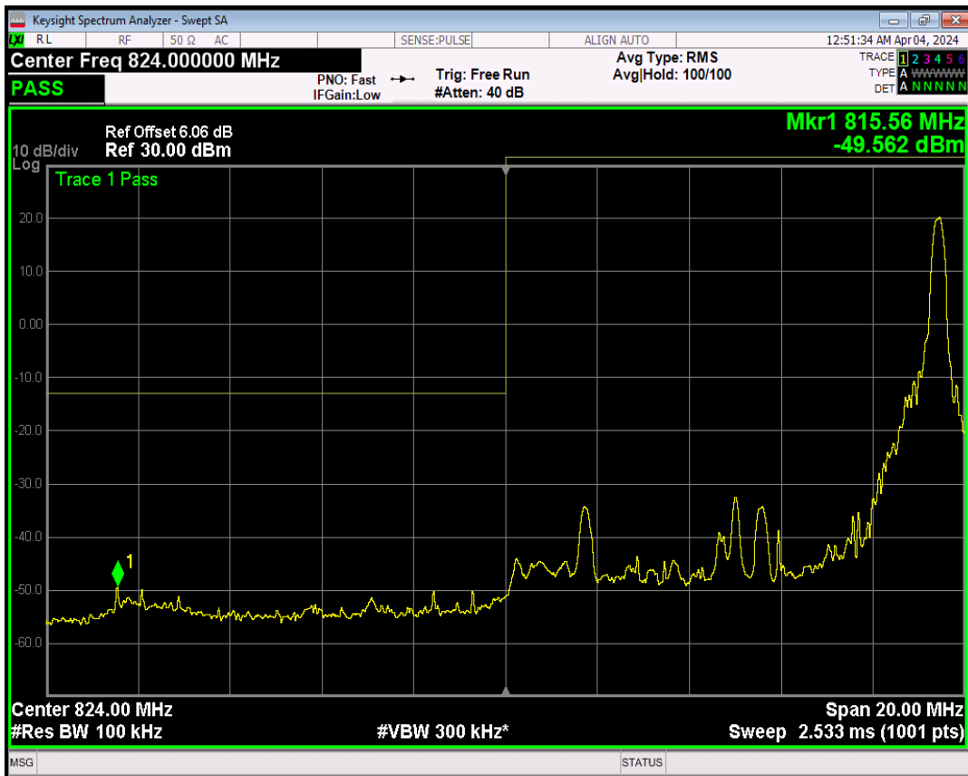
Band5 16QAM BW=10MHz Channel=20450 RB Size=50 Position=#0
