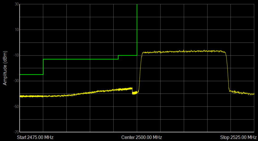
Band7 QPSK BW=20MHz Channel=20850 RB Size=100 Position=#0
