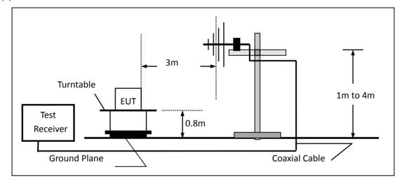
(c) For radiated emissions above 1000MHz
