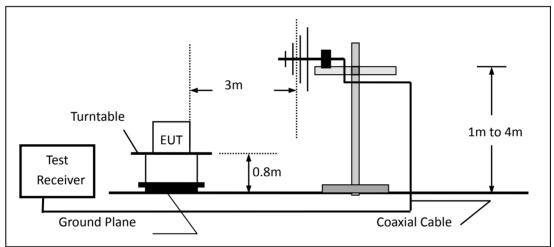
(c) For radiated emissions above 1000MHz
