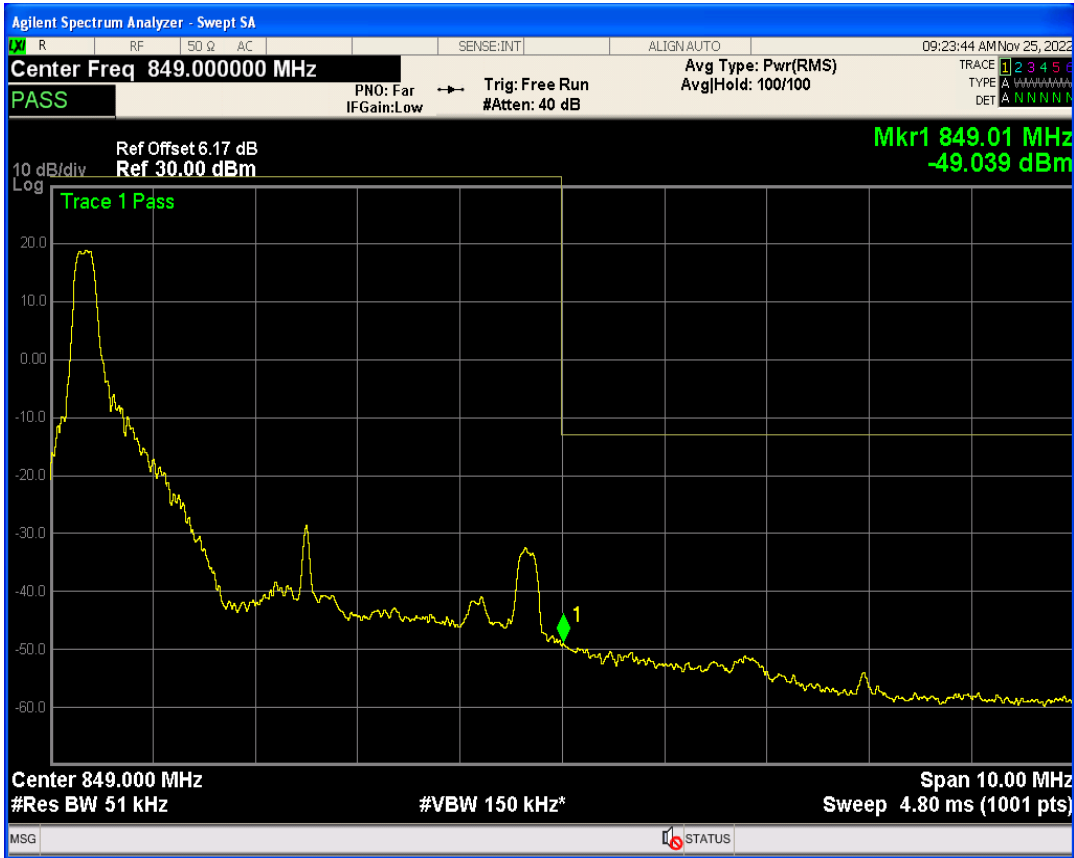
Band26b QPSK BW=5MHz Channel=27015 RB Size=1 Position=#Max
