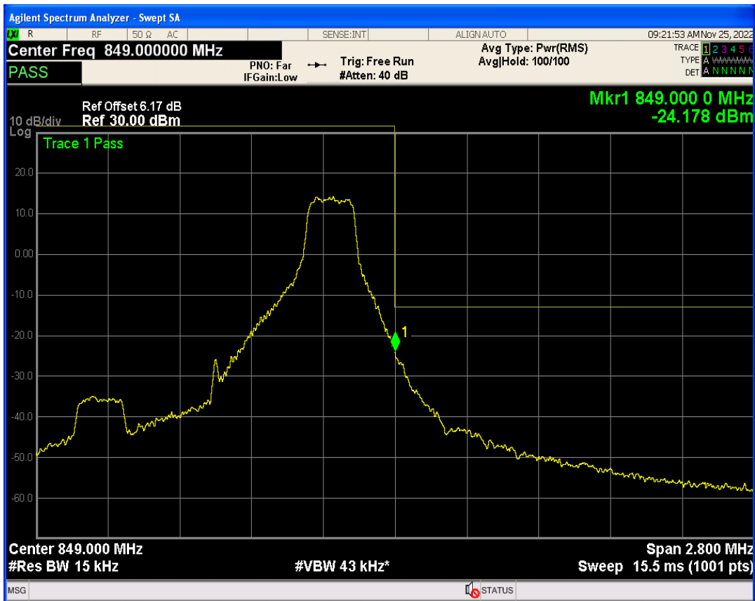
Band26b QPSK BW=1.4MHz Channel=27033 RB Size=6 Position=#0
