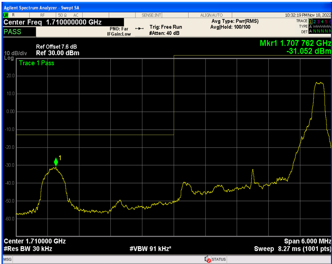
Band4 QAM16 BW=3MHz Channel=19965 RB Size=1 Position=#0
