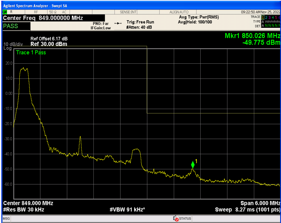
Band26b QPSK BW=3MHz Channel=27025 RB Size=1 Position=#Max
