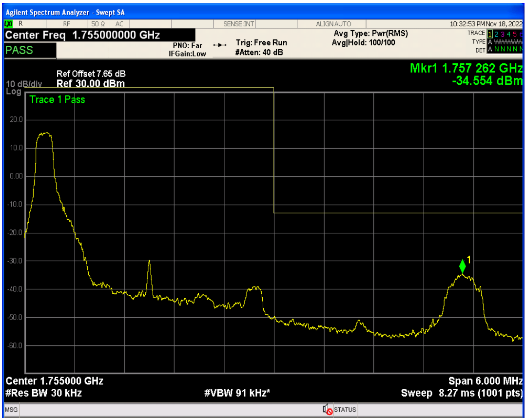
Band4 QAM16 BW=3MHz Channel=20385 RB Size=1 Position=#Max
