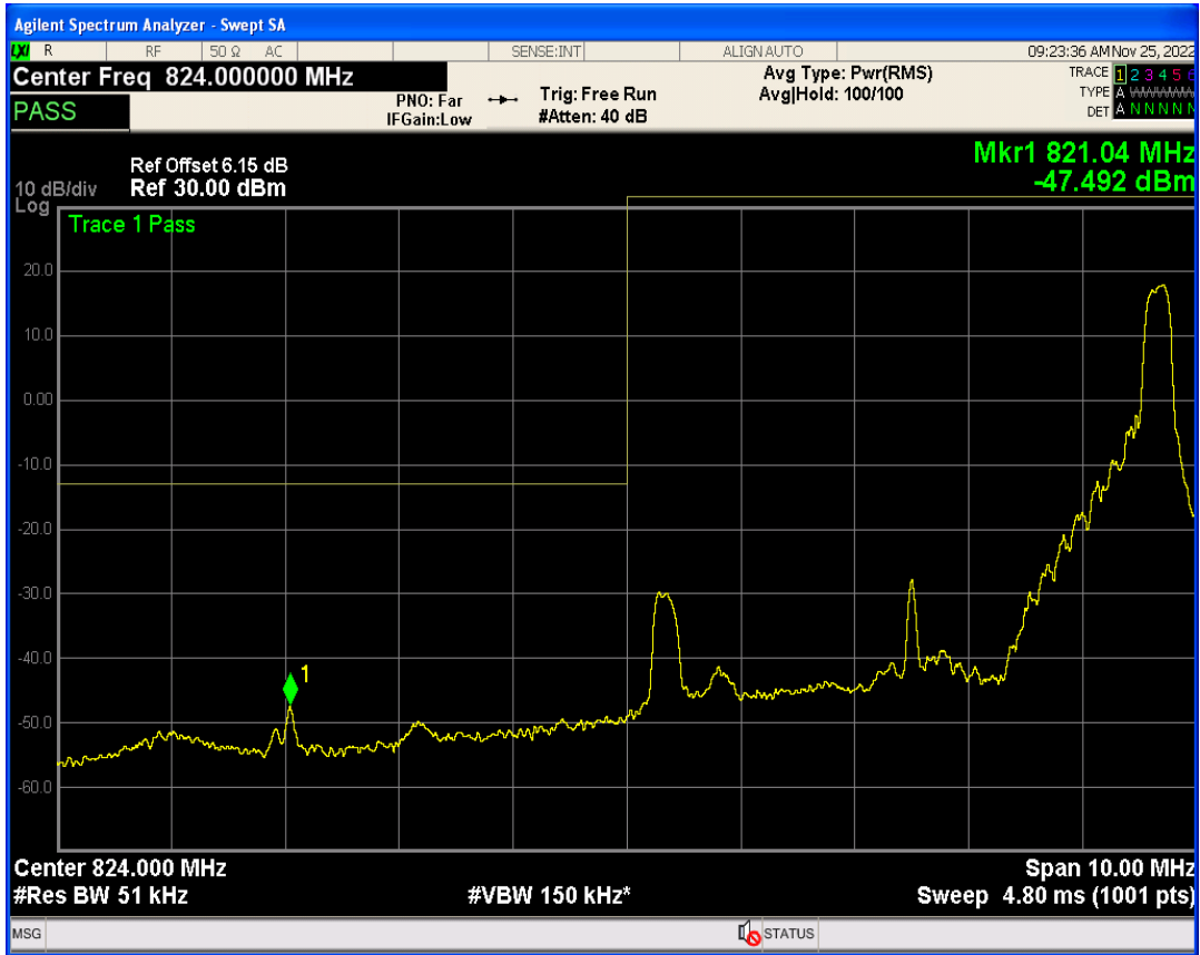
Band26b QAM16 BW=5MHz Channel=26815 RB Size=25 Position=#0
