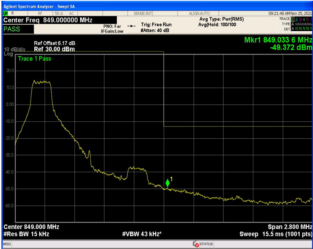
Band26b QPSK BW=1.4MHz Channel=27033 RB Size=1 Position=#Max
