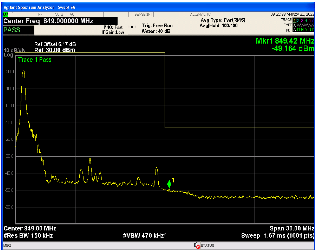
Band26b QAM16 BW=15MHz Channel=26965 RB Size=75 Position=#0
