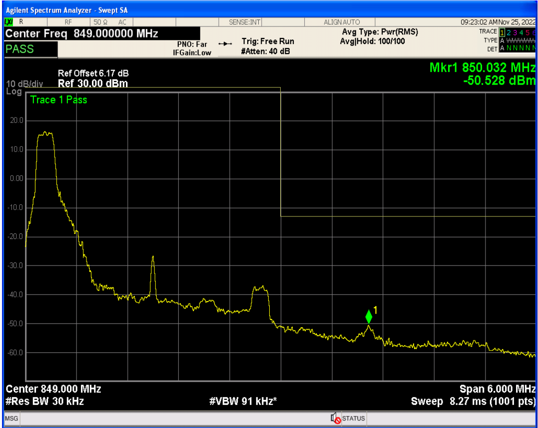
Band26b QPSK BW=5MHz Channel=26815 RB Size=1 Position=#0
