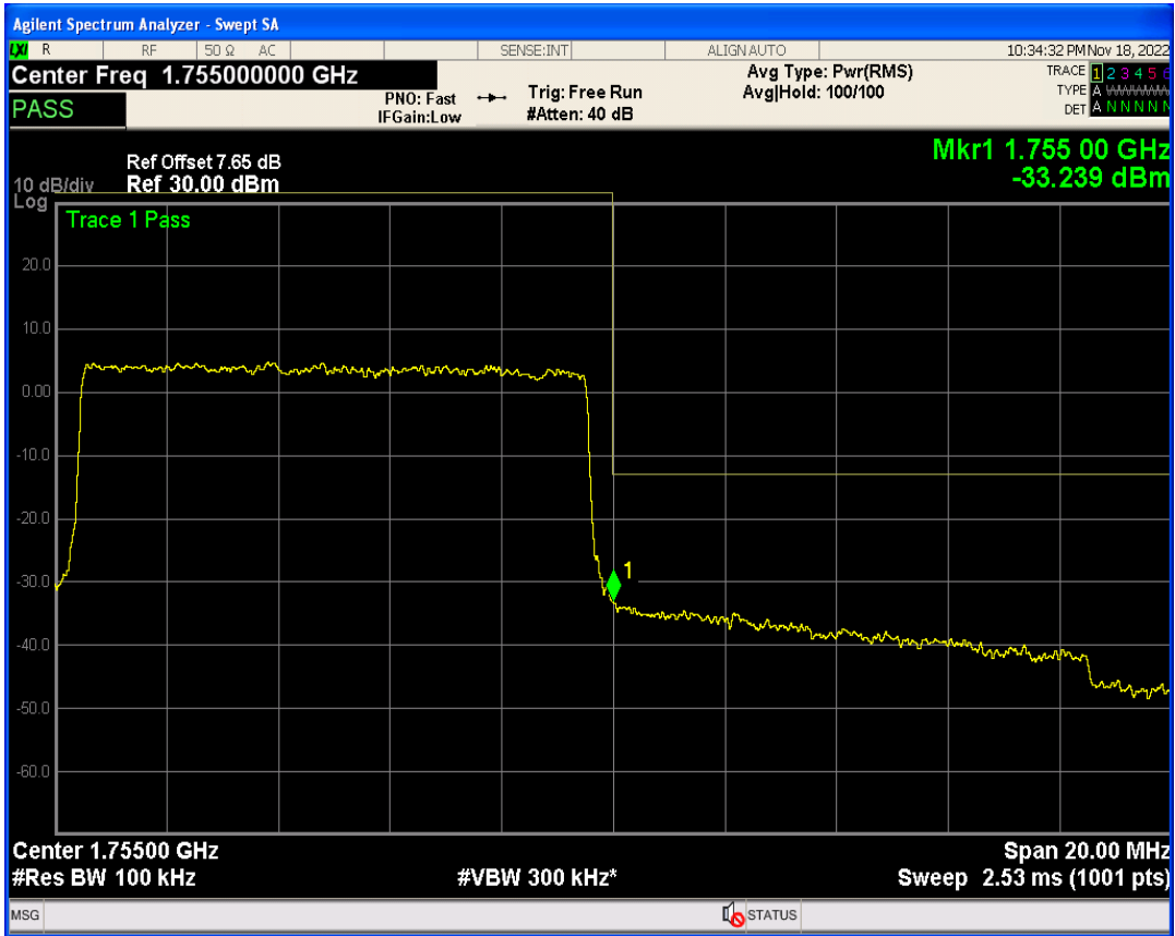
Band4 QAM16 BW=10MHz Channel=20350 RB Size=1 Position=#0
