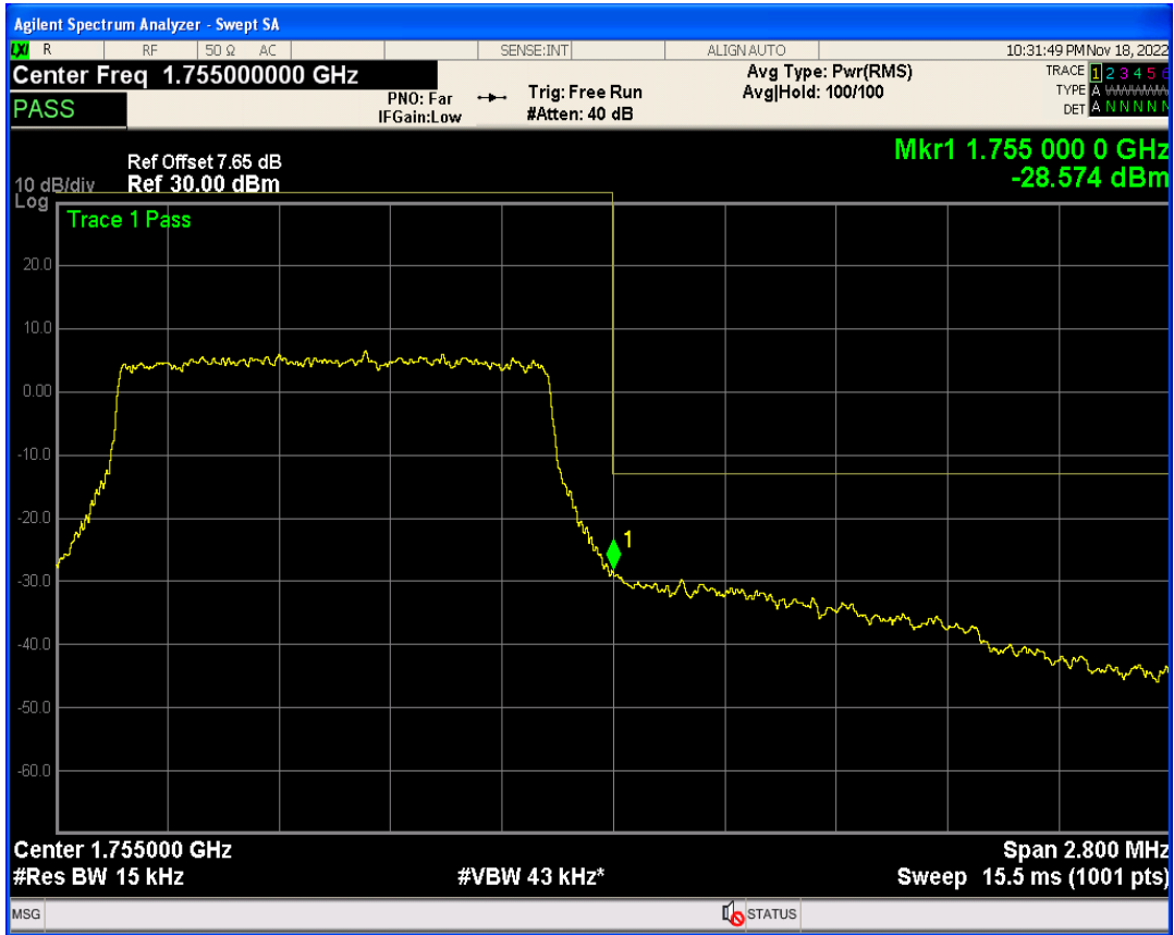
Band4 QAM16 BW=1.4MHz Channel=20393 RB Size=1 Position=#0
