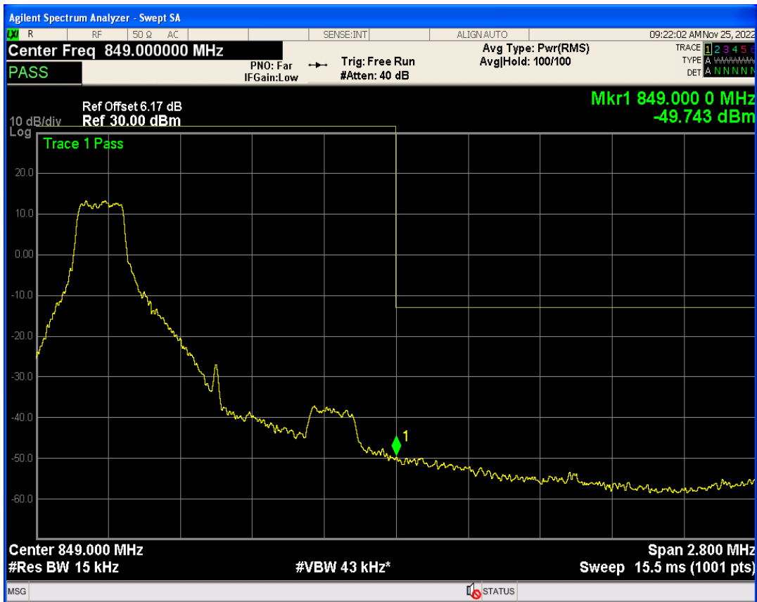
Band26b QAM16 BW=1.4MHz Channel=27033 RB Size=1 Position=#Max
