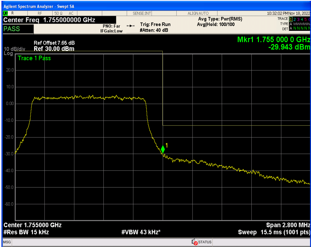
Band4 QPSK BW=3MHz Channel=19965 RB Size=1 Position=#Max
