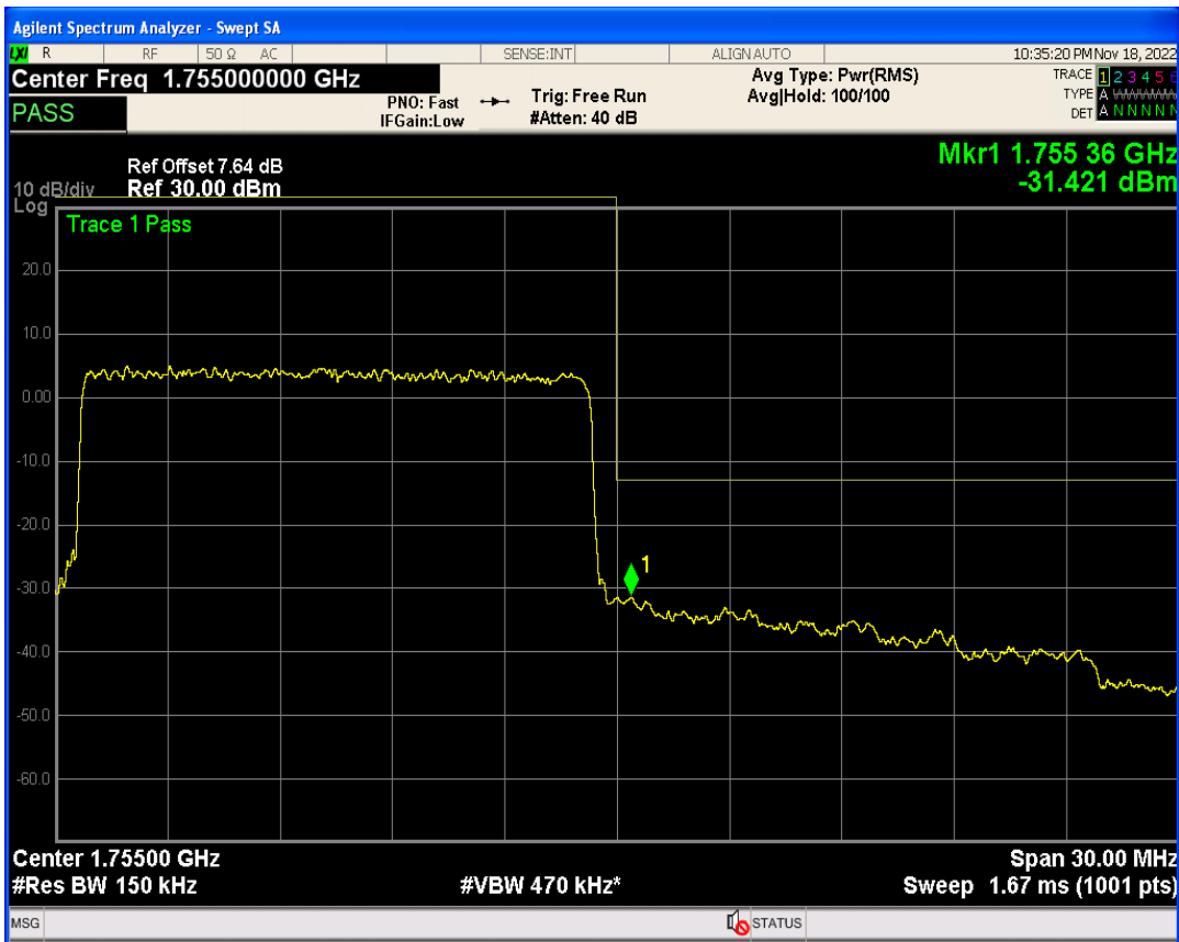
Band4 QAM16 BW=15MHz Channel=20325 RB Size=1 Position=#Max
