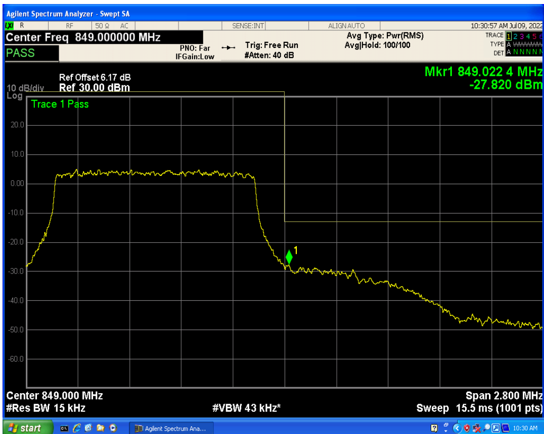
Band5 QAM16 BW=1.4MHz Channel=20643 RB Size=1 Position=#0
