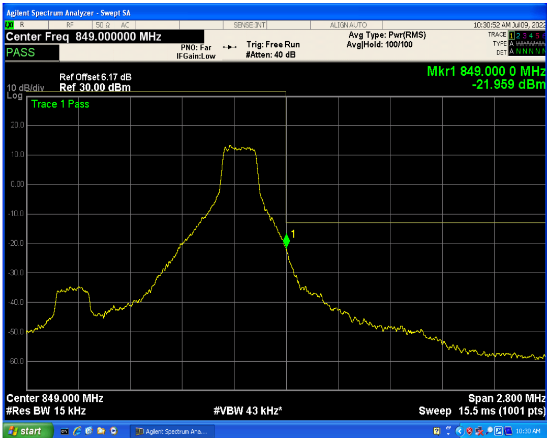
Band5 QPSK BW=1.4MHz Channel=20643 RB Size=6 Position=#0
