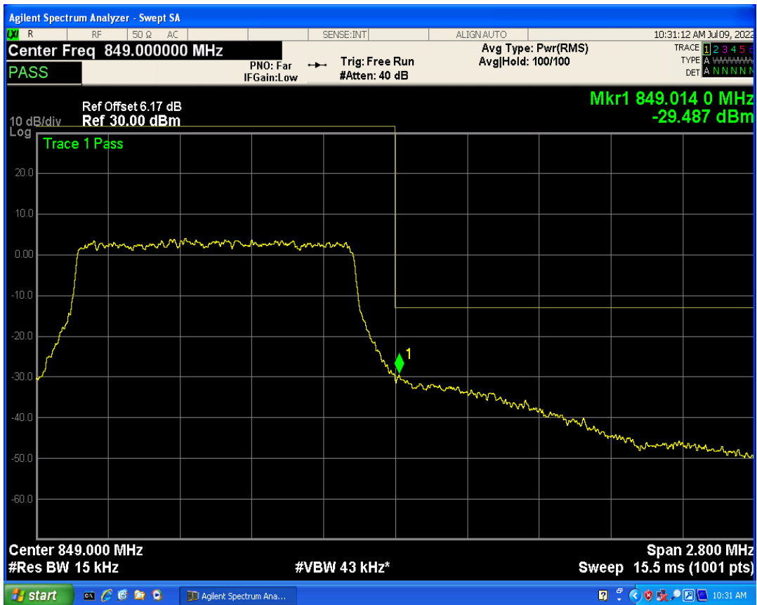
Band5 QPSK BW=3MHz Channel=20415 RB Size=1 Position=#0
