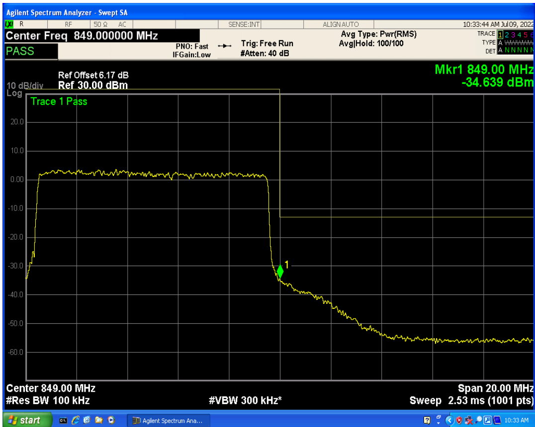
Band5 QAM16 BW=10MHz Channel=20600 RB Size=1 Position=#0
