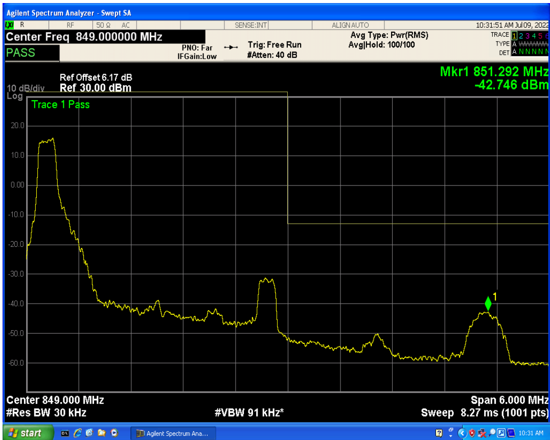
Band5 QAM16 BW=3MHz Channel=20415 RB Size=15 Position=#0
