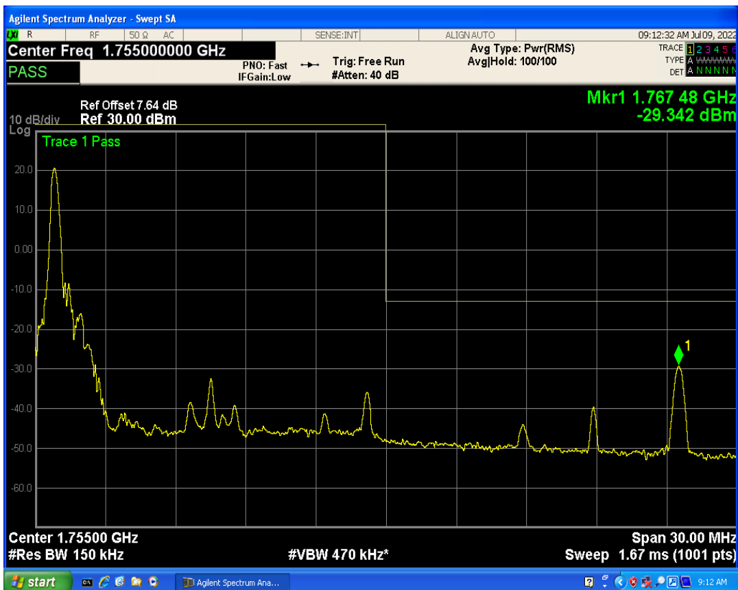
Band4 QPSK BW=15MHz Channel=20325 RB Size=75 Position=#0
