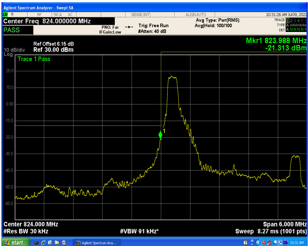
Band5 QPSK BW=3MHz Channel=20415 RB Size=15 Position=#0
