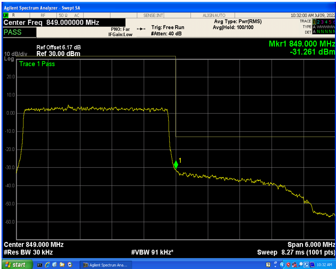
Band5 QAM16 BW=3MHz Channel=20635 RB Size=1 Position=#Max
