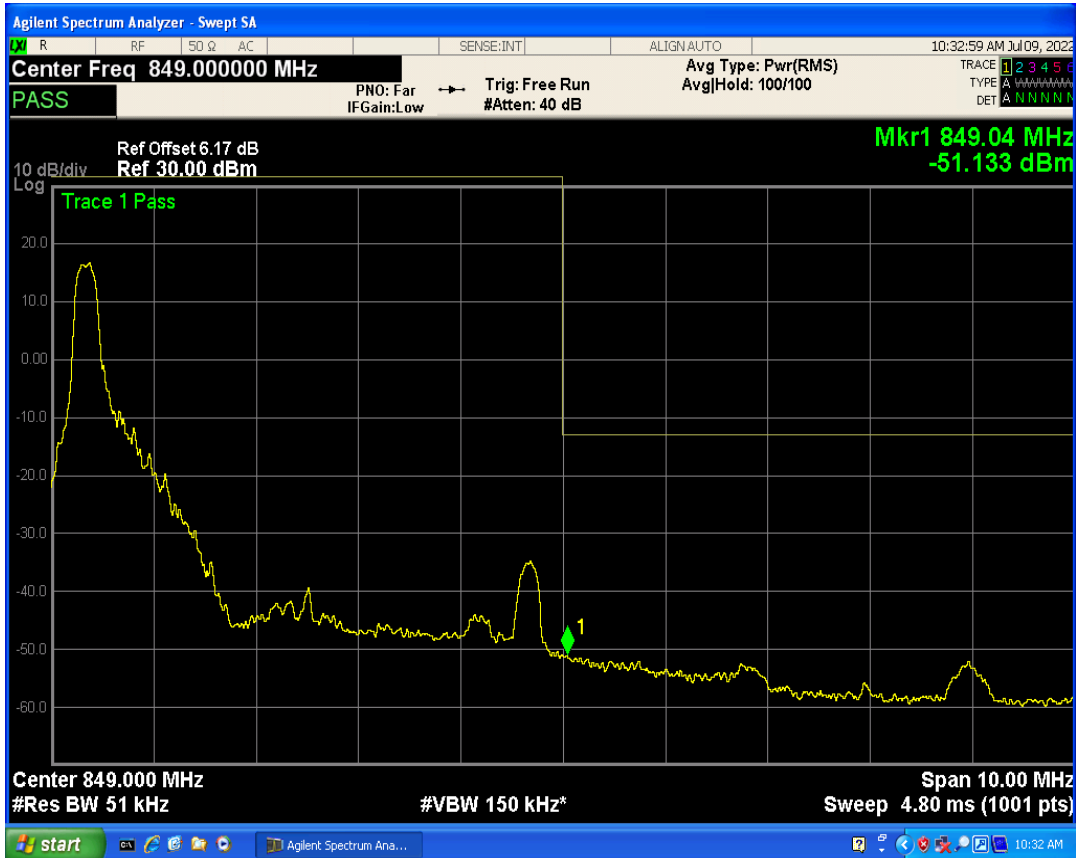
Band5 QAM16 BW=5MHz Channel=20625 RB Size=1 Position=#Max
