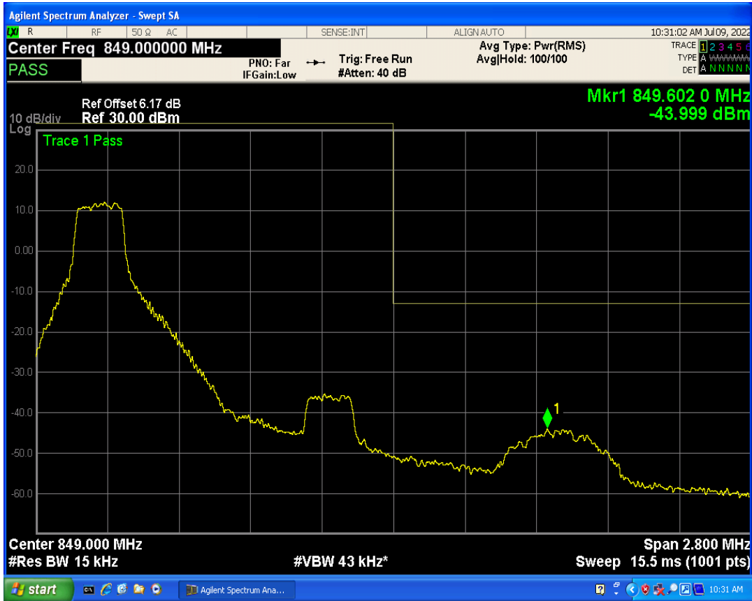
Band5 QAM16 BW=1.4MHz Channel=20643 RB Size=1 Position=#Max
