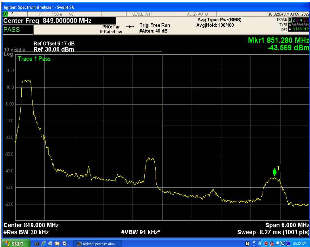
Band5 QPSK BW=3MHz Channel=20635 RB Size=15 Position=#0
