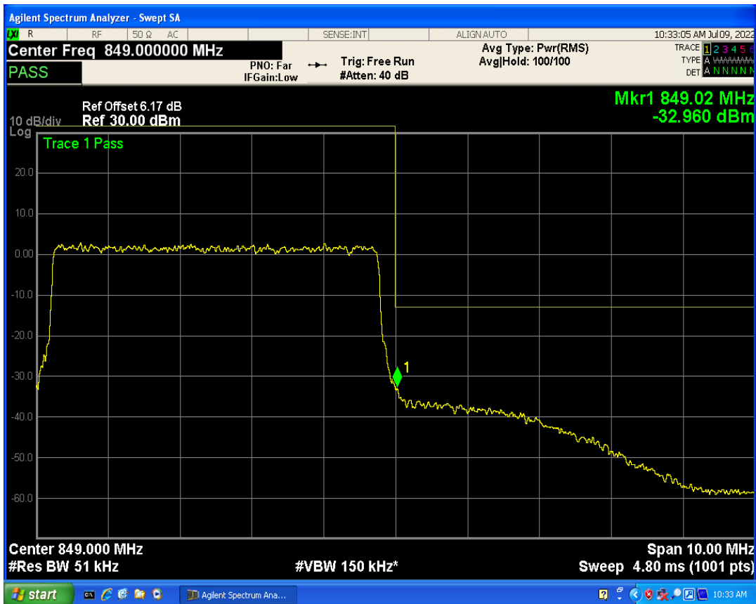
Band5 QPSK BW=10MHz Channel=20450 RB Size=1 Position=#Max
