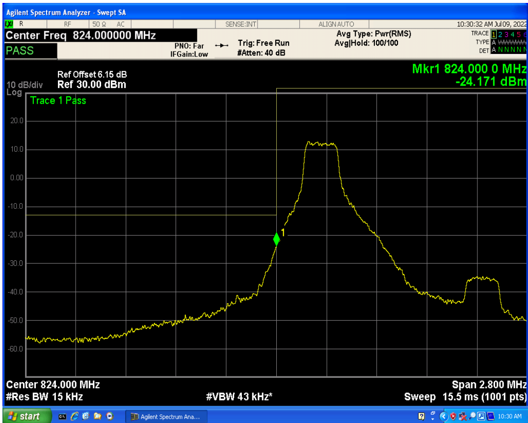
Band5 QAM16 BW=1.4MHz Channel=20407 RB Size=1 Position=#Max
