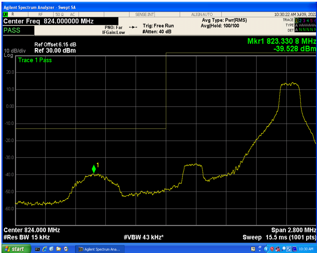
Band5 QPSK BW=1.4MHz Channel=20407 RB Size=6 Position=#0
