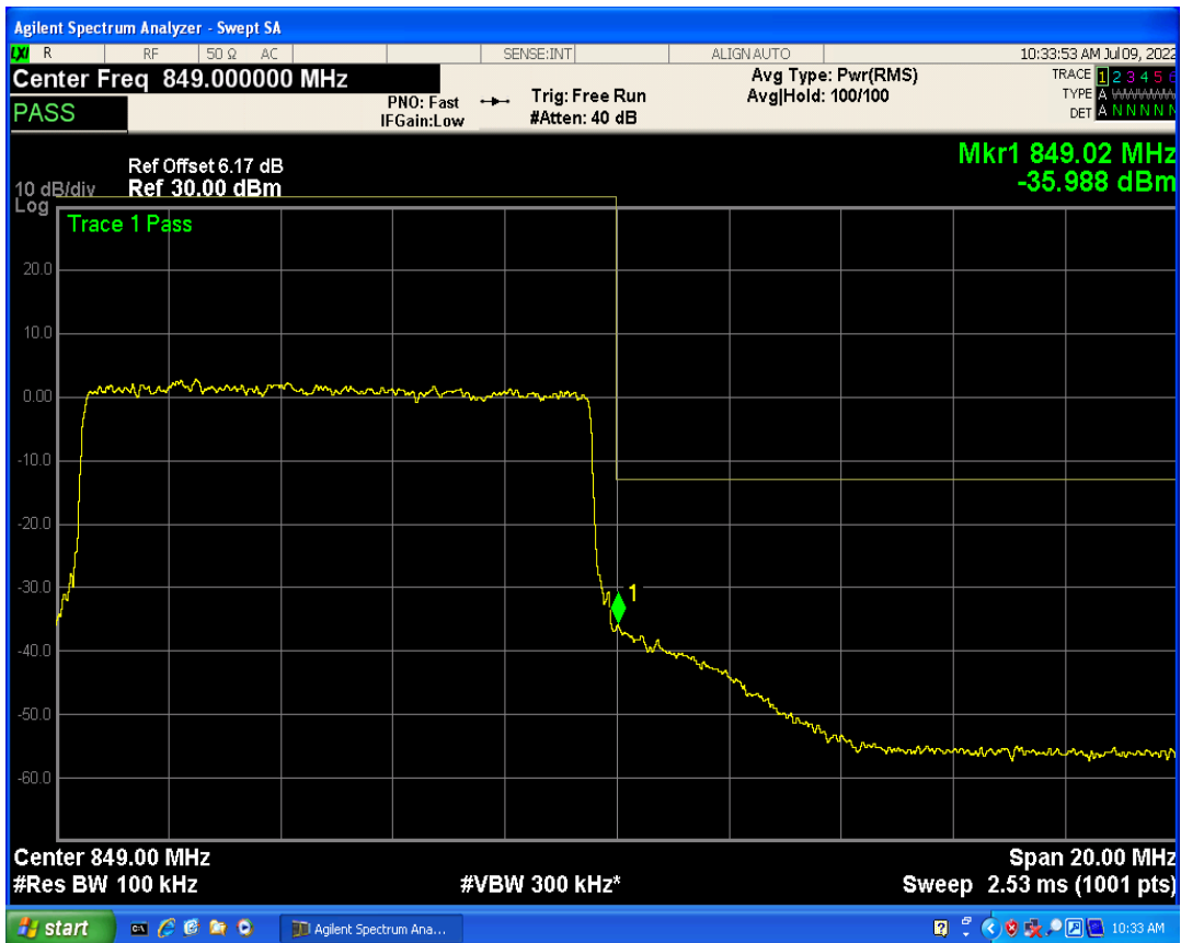
Band7 QPSK BW=5MHz Channel=20775 RB Size=1 Position=#0
