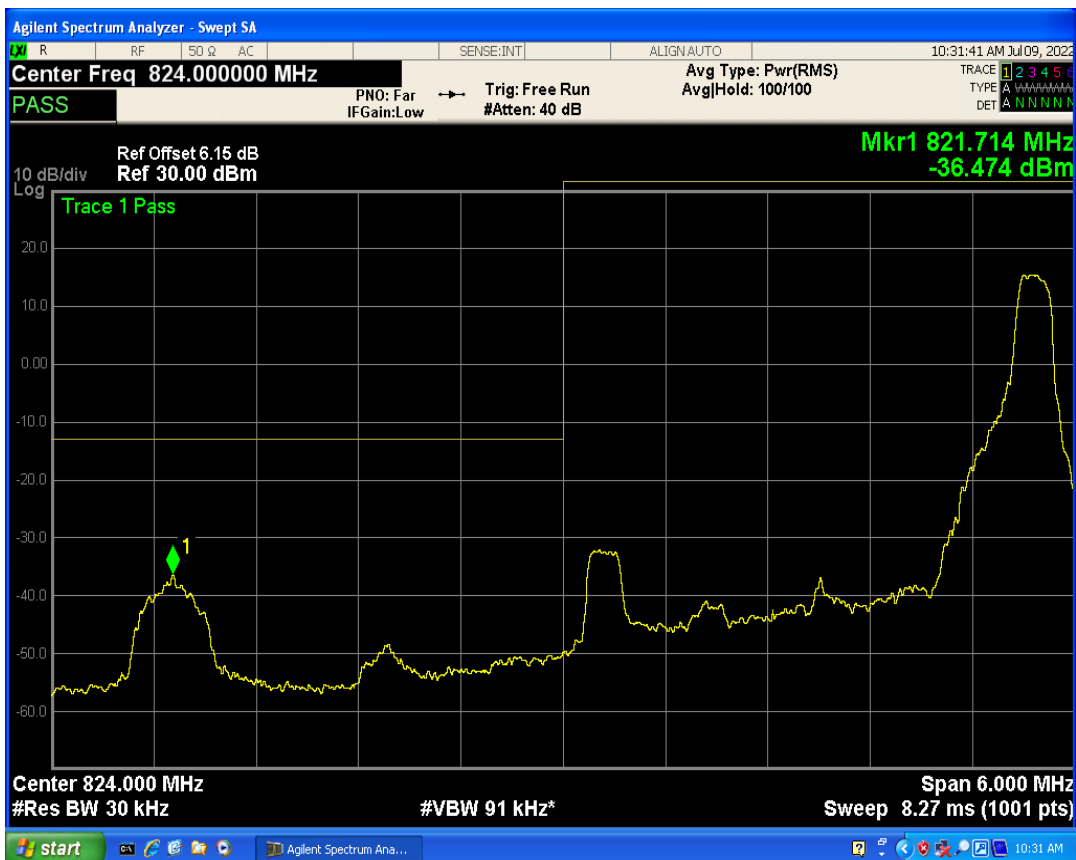
Band5 QPSK BW=3MHz Channel=20635 RB Size=1 Position=#0
