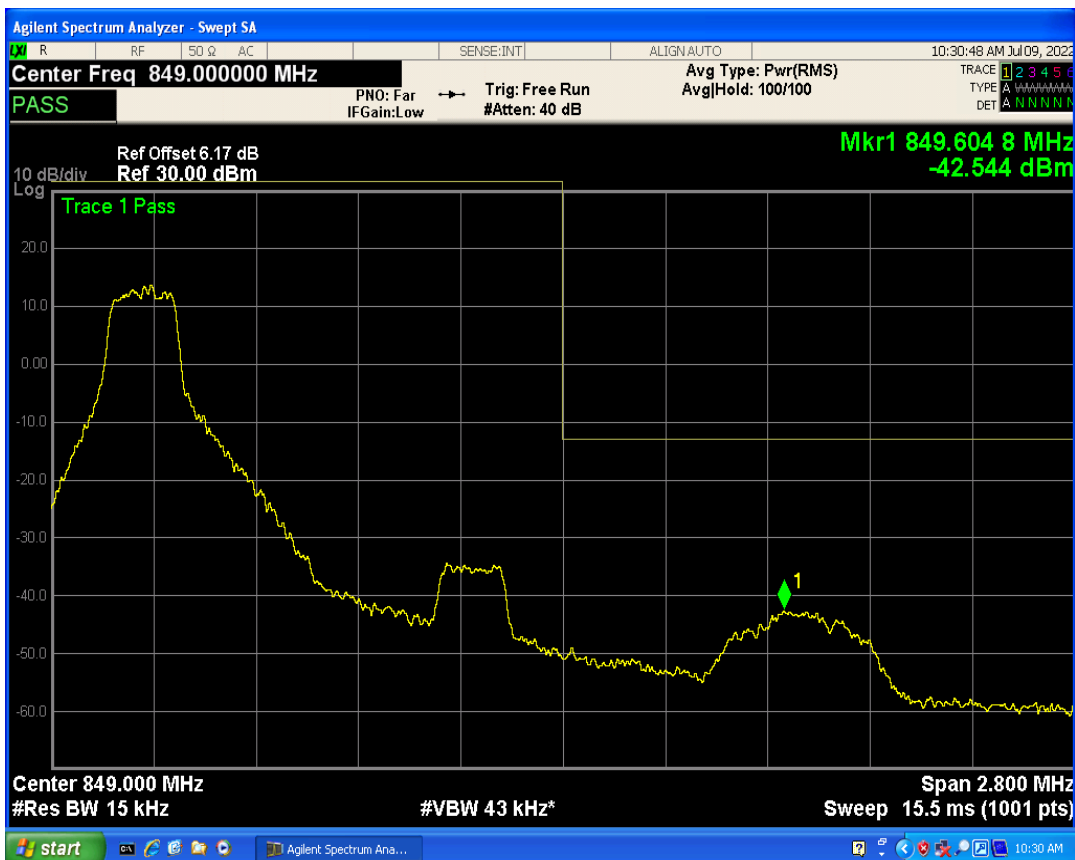
Band5 QPSK BW=1.4MHz Channel=20643 RB Size=1 Position=#Max
