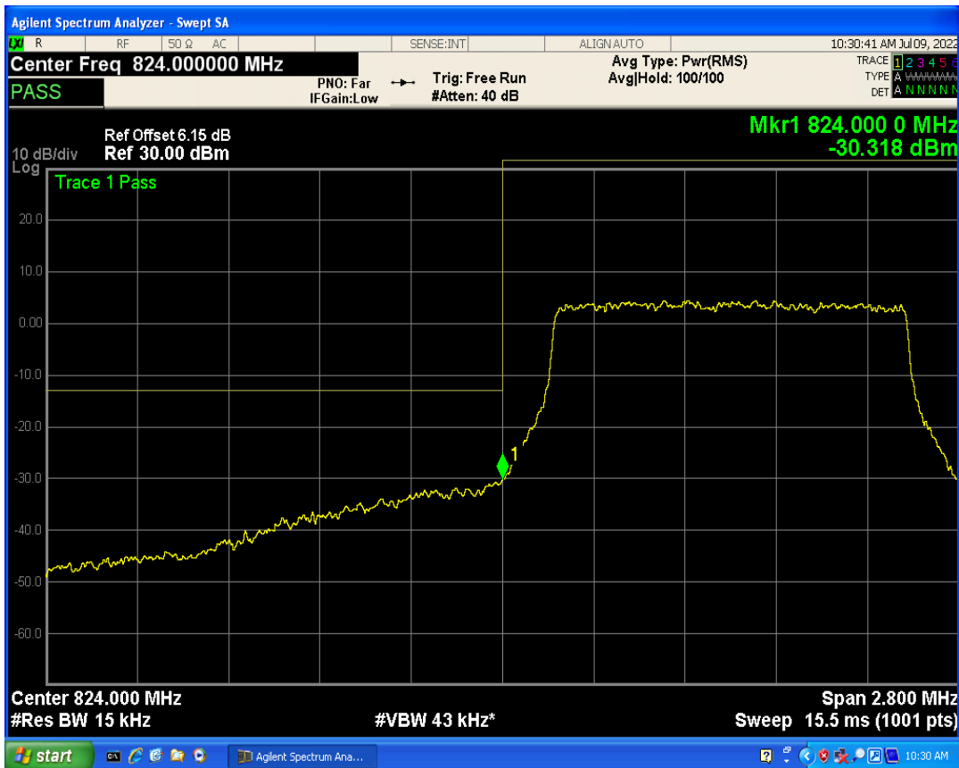
Band5 QPSK BW=1.4MHz Channel=20643 RB Size=1 Position=#0
