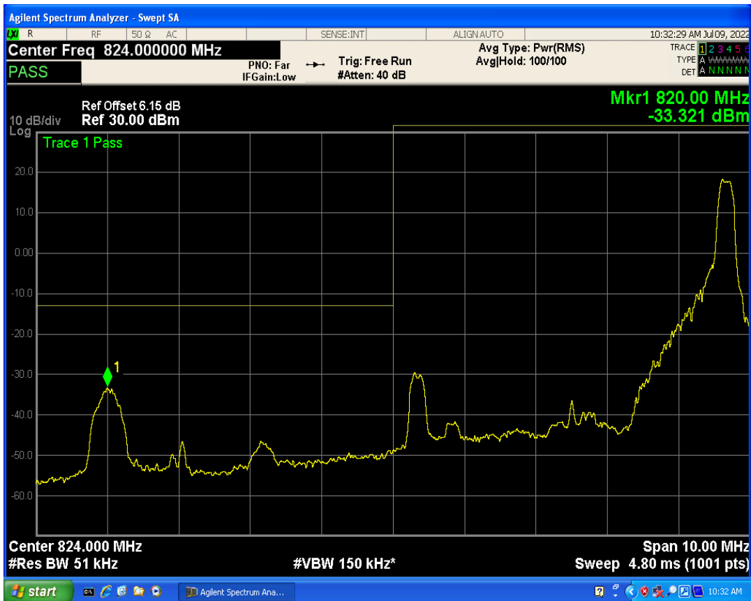
Band5 QPSK BW=5MHz Channel=20425 RB Size=25 Position=#0
