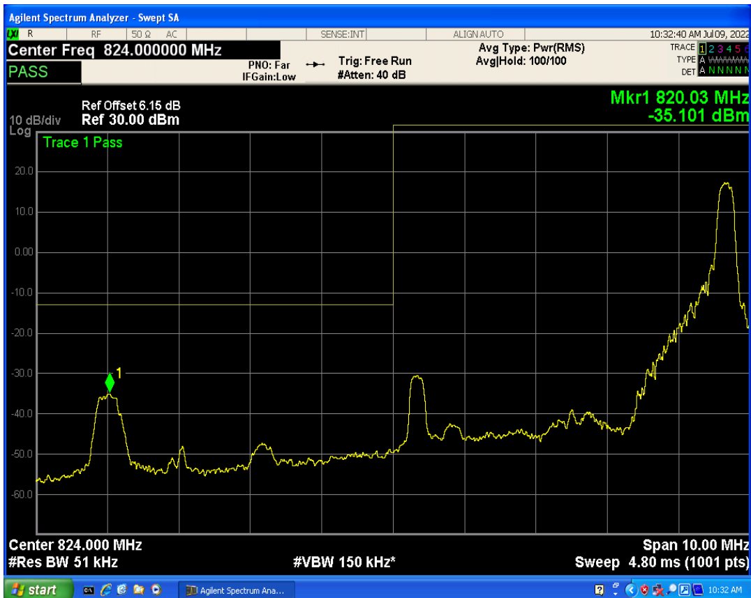
Band5 QAM16 BW=5MHz Channel=20425 RB Size=25 Position=#0
