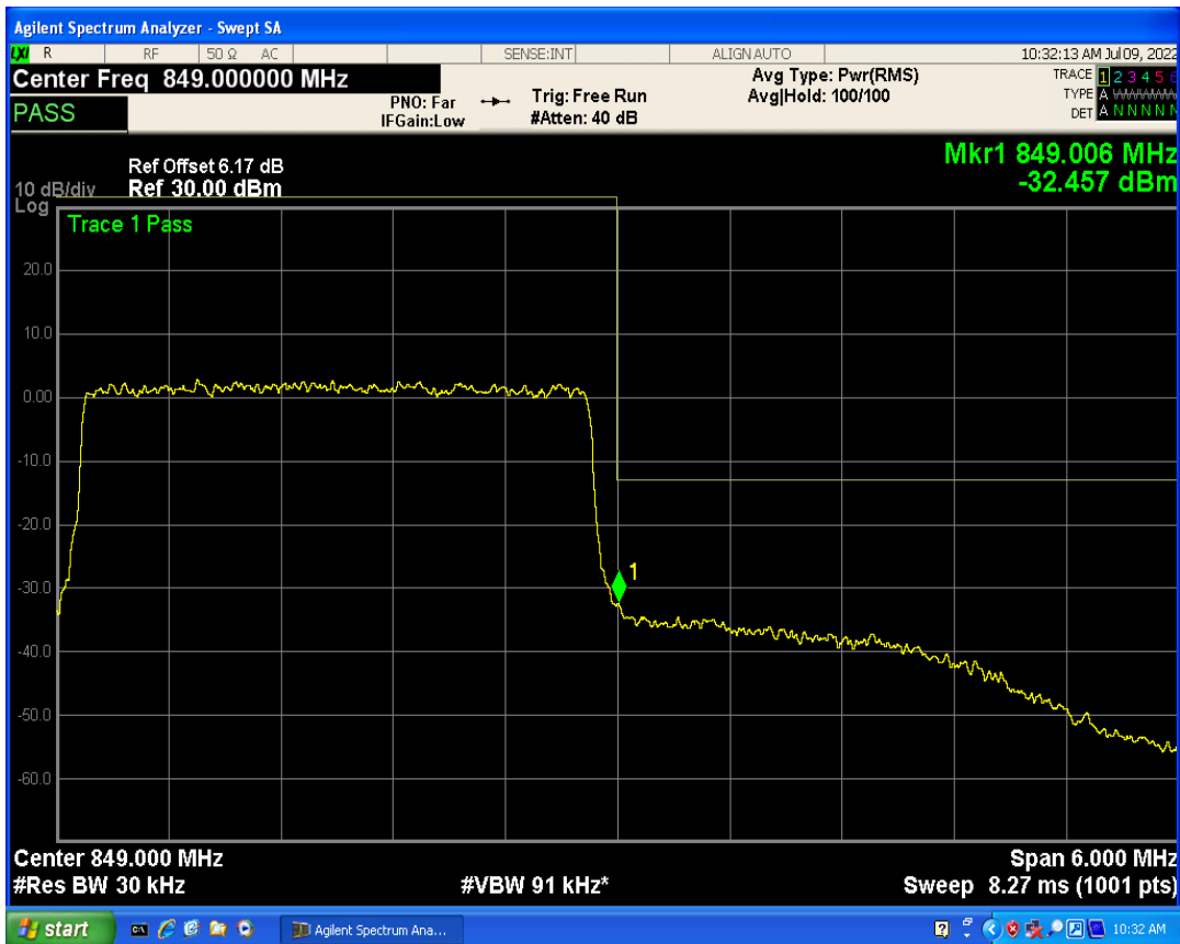
Band5 QPSK BW=5MHz Channel=20425 RB Size=1 Position=#0
