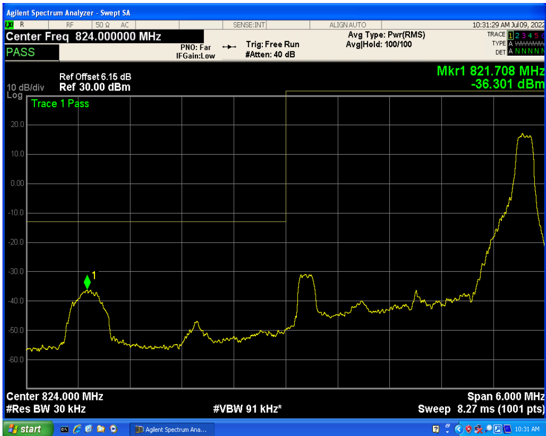
Band5 QAM16 BW=3MHz Channel=20415 RB Size=1 Position=#0
