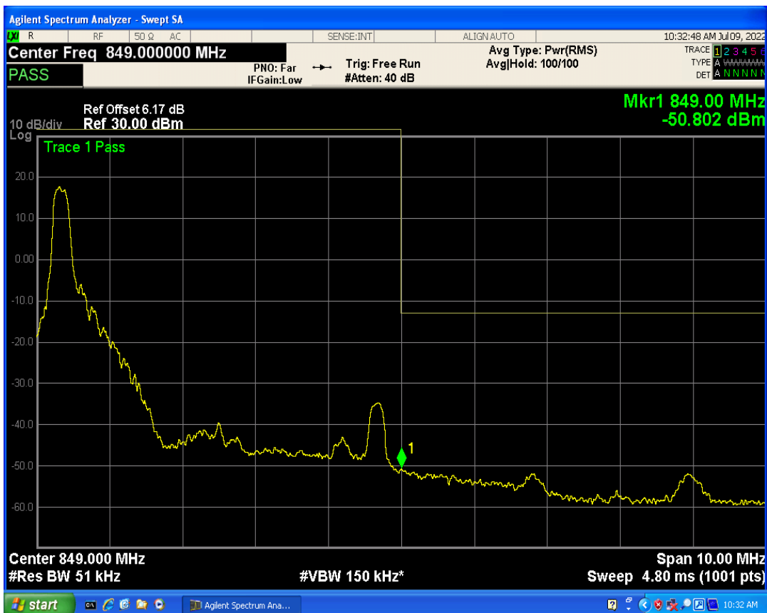
Band5 QPSK BW=5MHz Channel=20625 RB Size=1 Position=#Max
