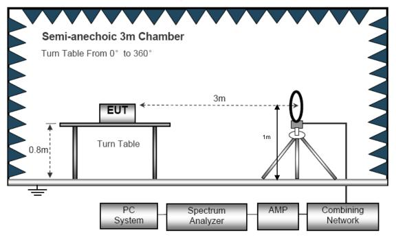
(B) Radiated Emission Test-Up Frequency 30MHz~1GHz
