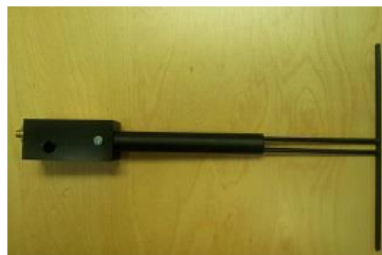
Figure 1 – MVG COMOSAR Validation Dipole
