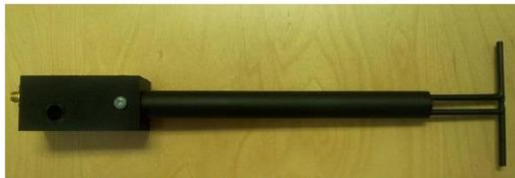
Figure 1 – MVG COMOSAR Validation Dipole
