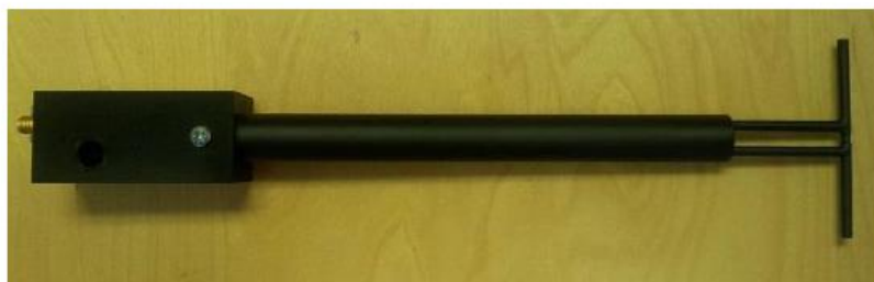
Figure 1 – MVG COMOSAR Validation Dipole
