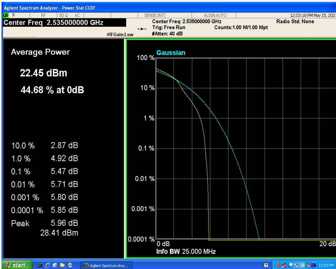
Band7 QPSK BW=20MHz Channel=21100 RB Size=1 Position=#0
