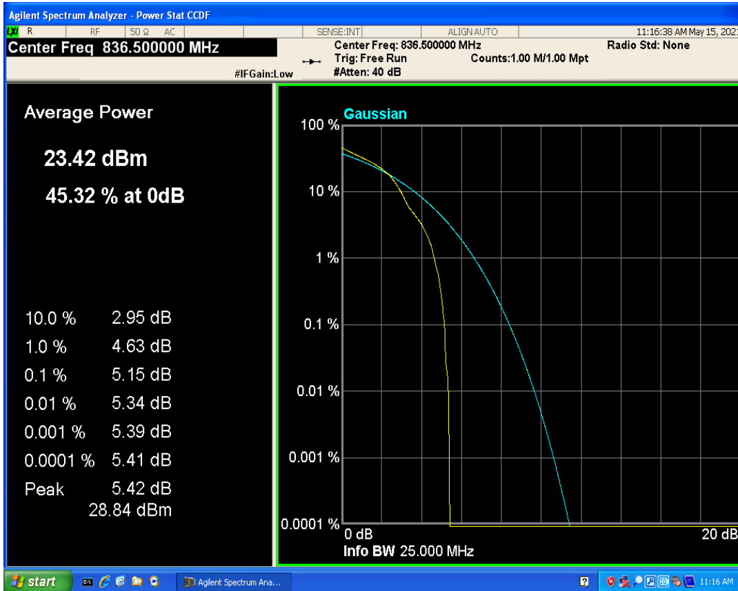
Band5 QPSK BW=3MHz Channel=20525 RB Size=1 Position=#0
