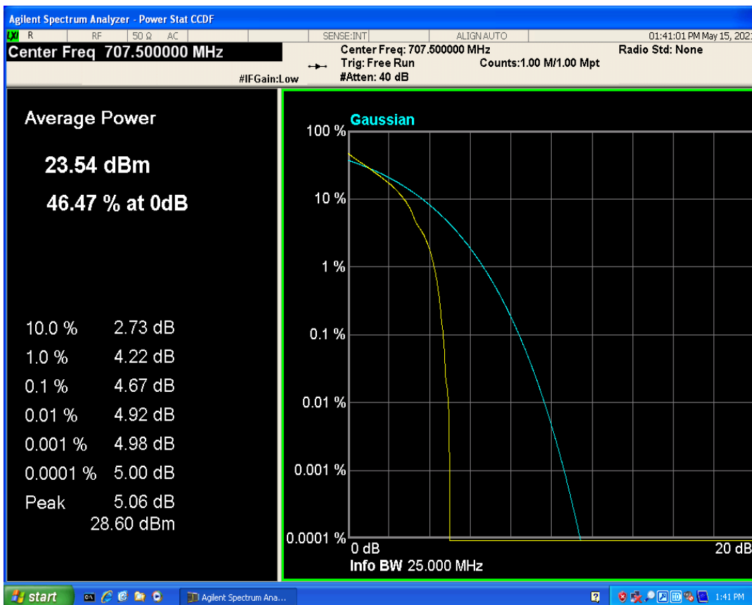
Band12 QAM16 BW=3MHz Channel=23095 RB Size=1 Position=#0
