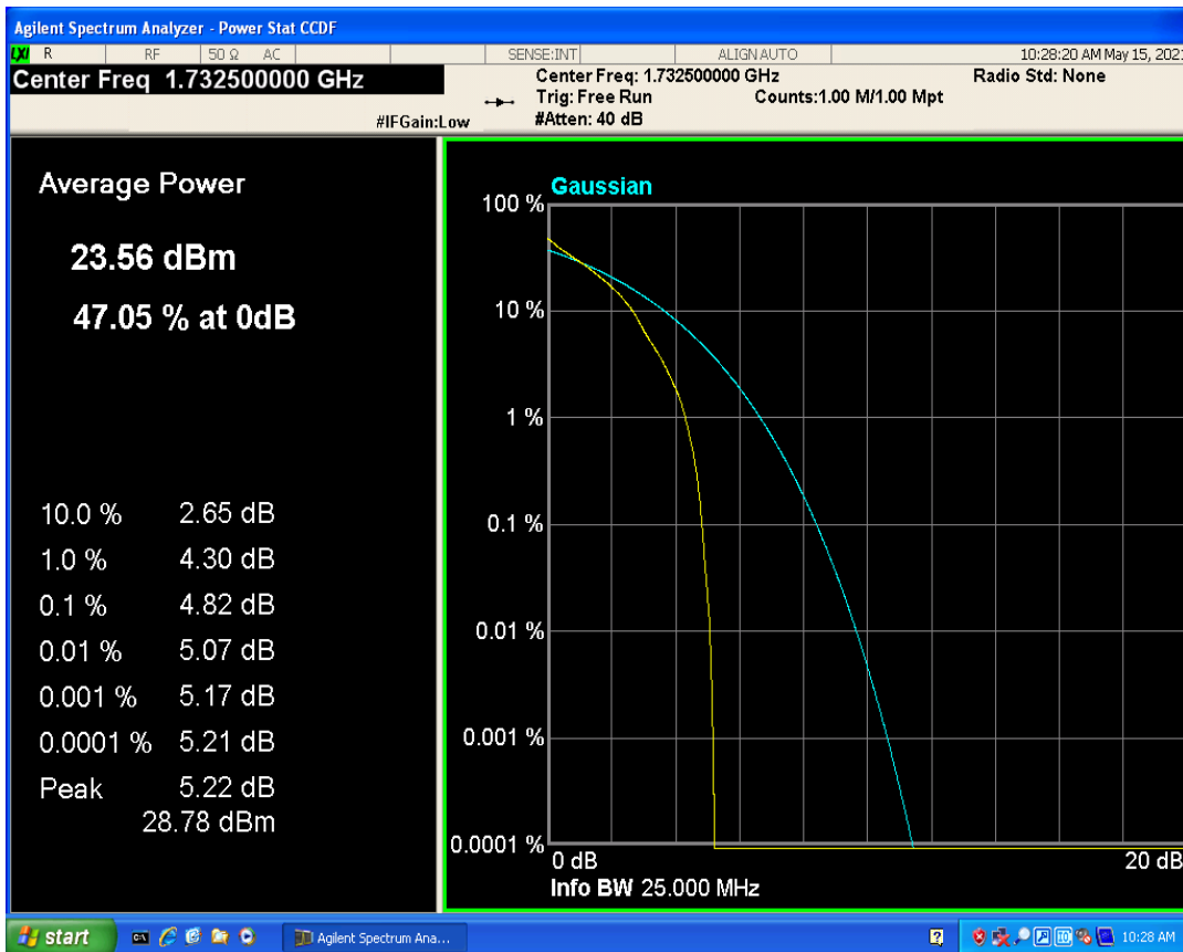
Band5 QPSK BW=1.4MHz Channel=20525 RB Size=1 Position=#0
