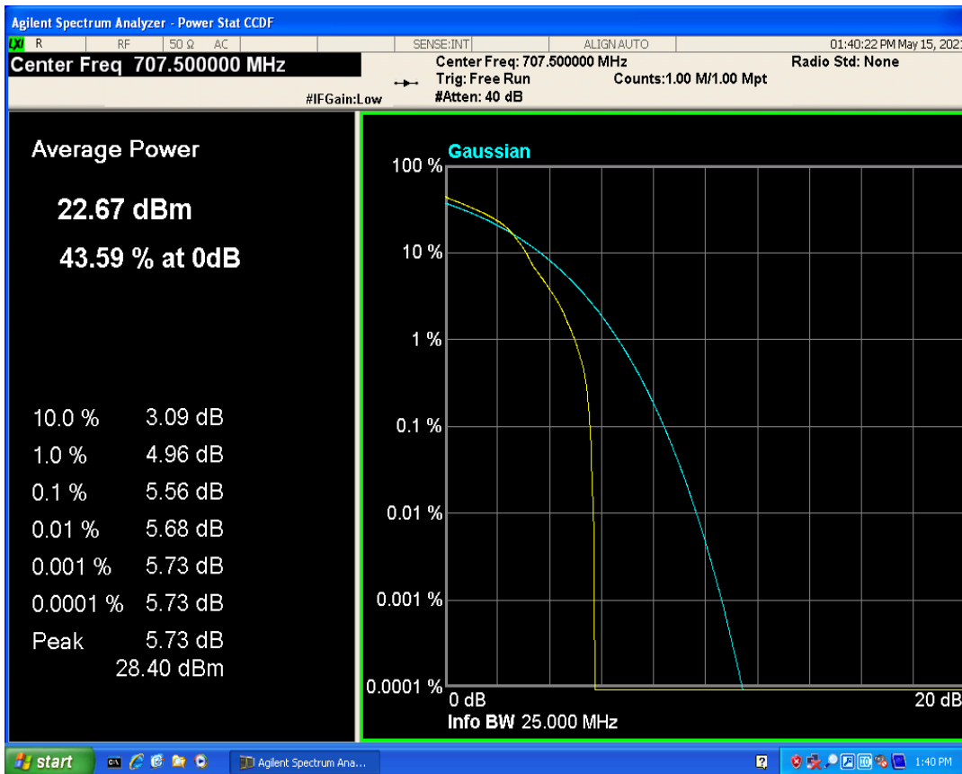
Band12 QPSK BW=3MHz Channel=23095 RB Size=1 Position=#0
