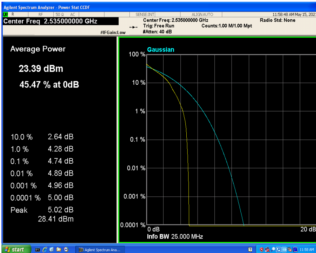
Band7 QPSK BW=15MHz Channel=21100 RB Size=1 Position=#0
