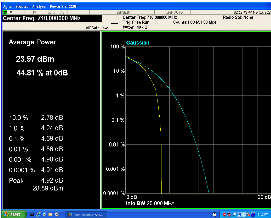
Band17 QPSK BW=10MHz Channel=23790 RB Size=1 Position=#0
