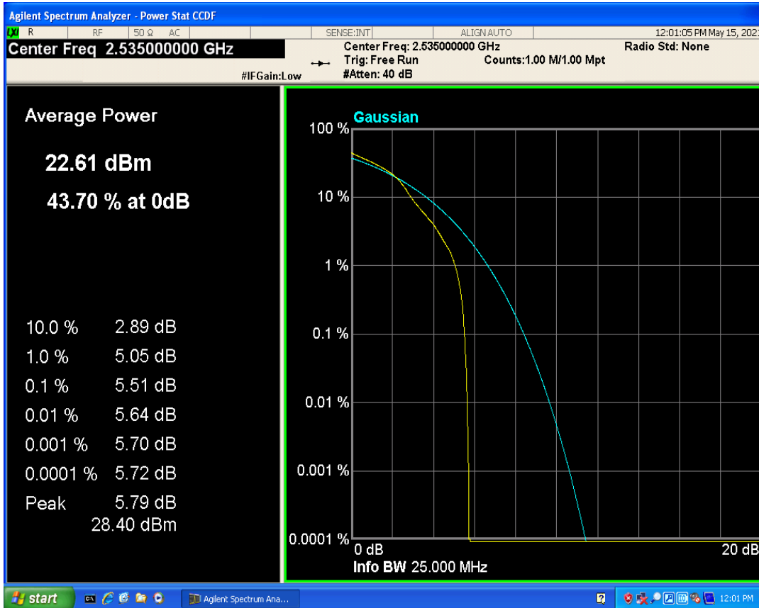
Band7 QAM16 BW=20MHz Channel=21100 RB Size=1 Position=#0
