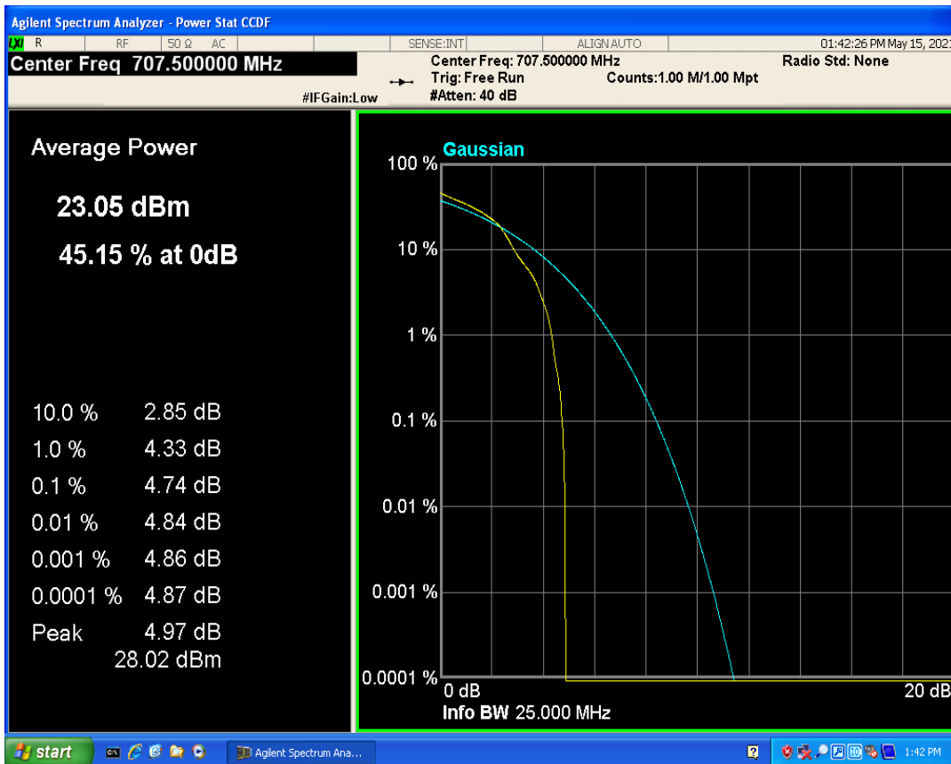
Band12 QPSK BW=10MHz Channel=23095 RB Size=1 Position=#0
