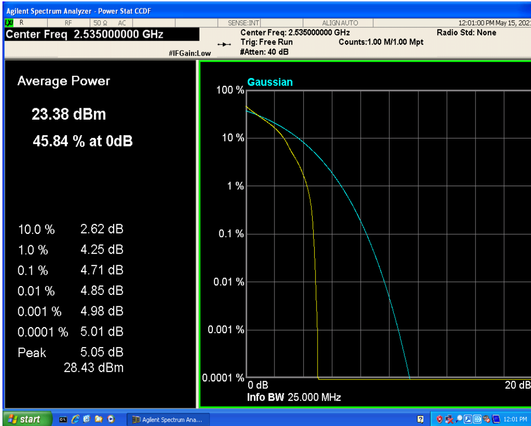
Band7 QAM16 BW=10MHz Channel=21100 RB Size=1 Position=#0
