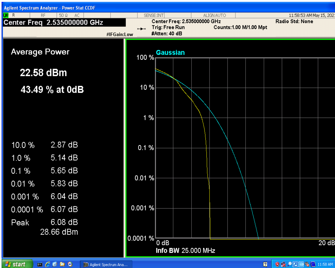
Band7 QAM16 BW=15MHz Channel=21100 RB Size=1 Position=#0
