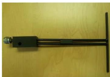
Figure 1 – MVG COMOSAR Validation Dipole
