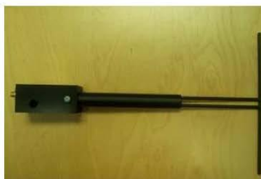
Figure 1 – MVG COMOSAR Validation Dipole
