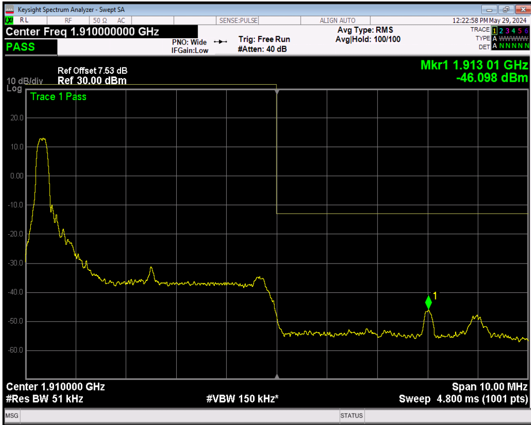
Band2 QPSK BW=5MHz Channel=19175 RB Size=1 Position=#Max
