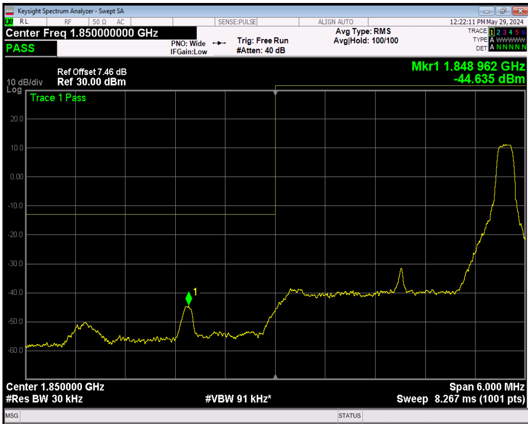
Band2 QPSK BW=3MHz Channel=18615 RB Size=15 Position=#0
