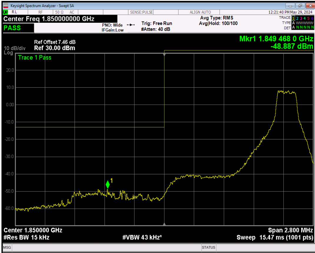
Band2 16QAM BW=1.4MHz Channel=18607 RB Size=6 Position=#0
