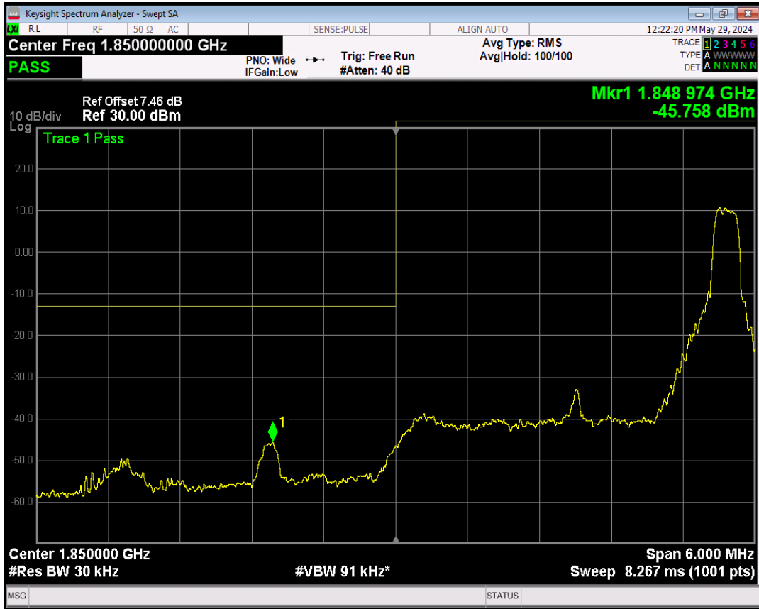
Band2 16QAM BW=3MHz Channel=18615 RB Size=15 Position=#0
