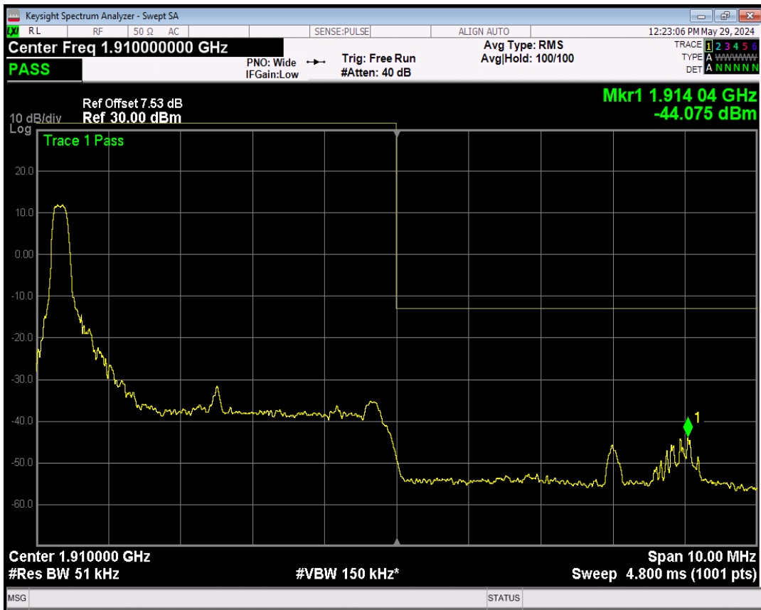
Band2 16QAM BW=5MHz Channel=19175 RB Size=1 Position=#Max
