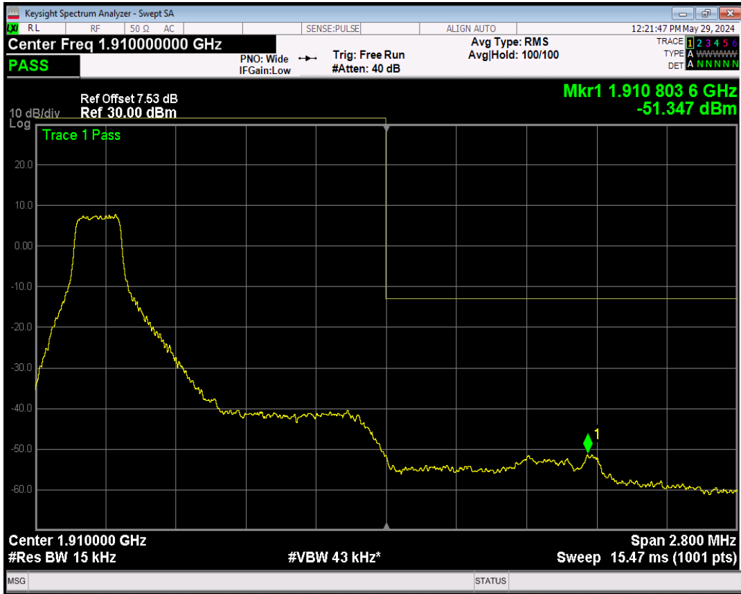
Band2 QPSK BW=1.4MHz Channel=19193 RB Size=1 Position=#Max
