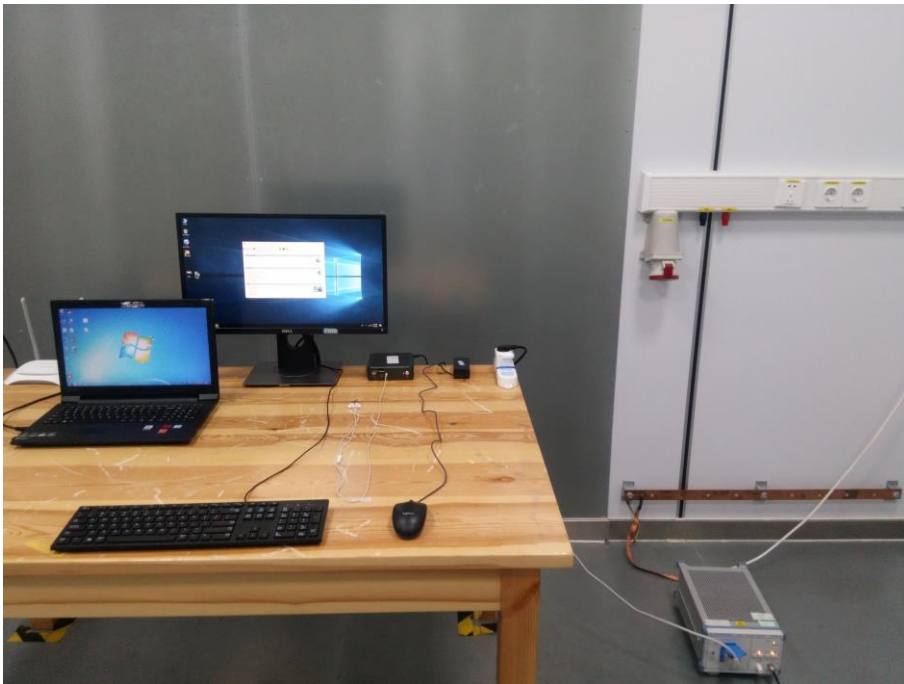
Fig. 4 Power line conducted emission setup photo
