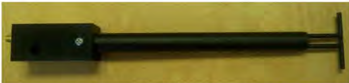
Figure 1 – MVG COMOSAR Validation Dipole
