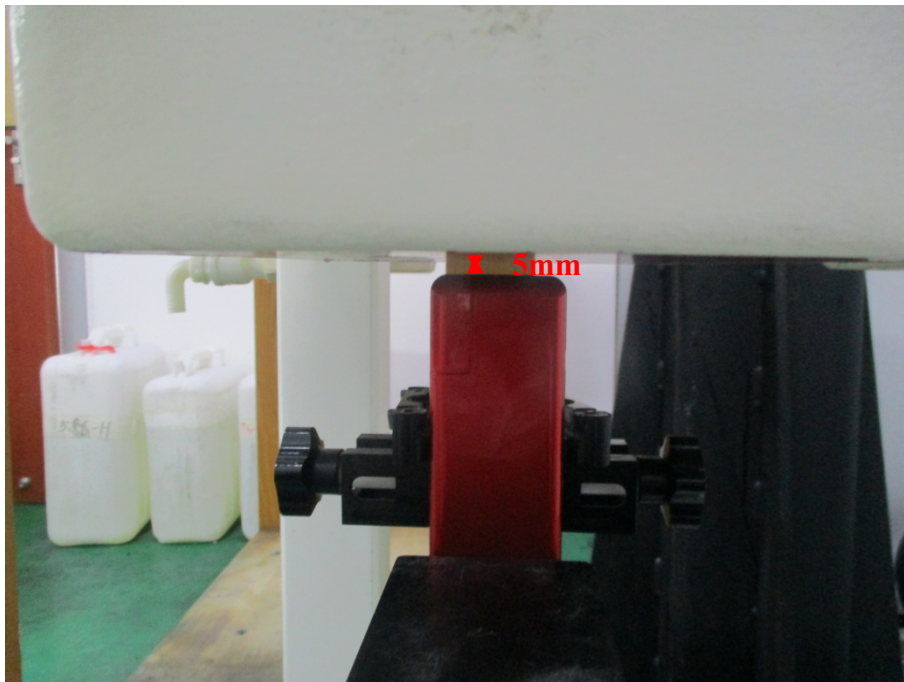
Body Bottom Setup Photo (5mm)
